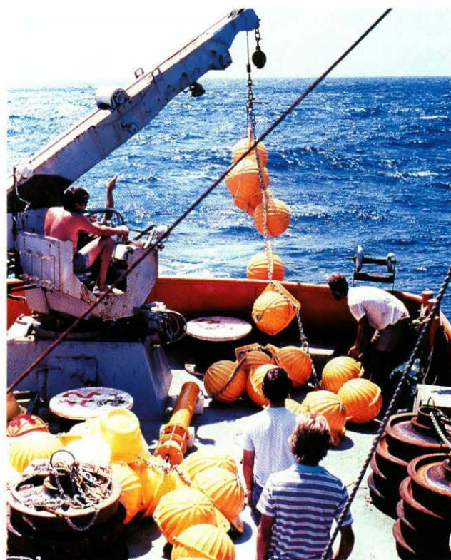
An array of current meters being launched from LONGHORN off the continental slope. Yellow "hardhats" protect glass flotation spheres and railroad wheels anchor the arrays to the ocean floor via acoustic releases.
