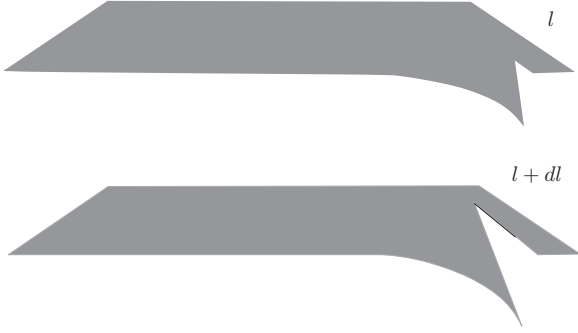
FIG. 4. (Top) Clamped, free-standing two-dimensional sheet with an initial crack of length l at the right-hand side. The sheet is clamped at the left and right edges. (Bottom) Because of an external downward force, the crack runs a length dl , and the sheet bends diagonally.
