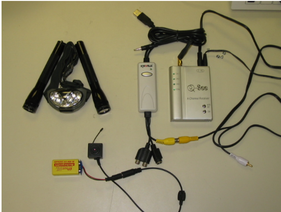
Figure 3.32. Hardware needed for image acquisition using on-board camera. Shown in the picture are (from left to right) the flashlights and headlight, DVD Maker USB2.0 Capture Box, Q-See 4-Channel Receiver, and Q-See 2.4 GHz Wireless Camera (bottom).
