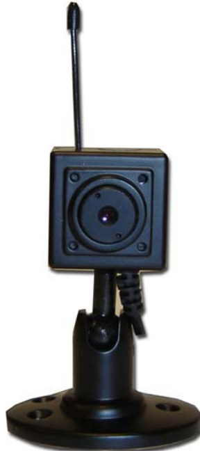
Figure 3.4. Q-See QSWMC 2.4 GHz Wireless Camera used as on-board camera.
