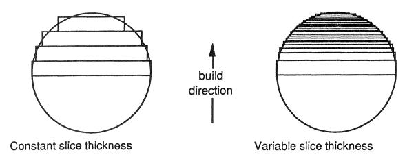
Figure 4. Effect of variable slice thickness on part accuracy.
