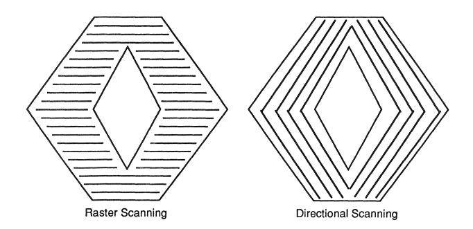
Figure 5. Directional scanning versus raster scanning.
