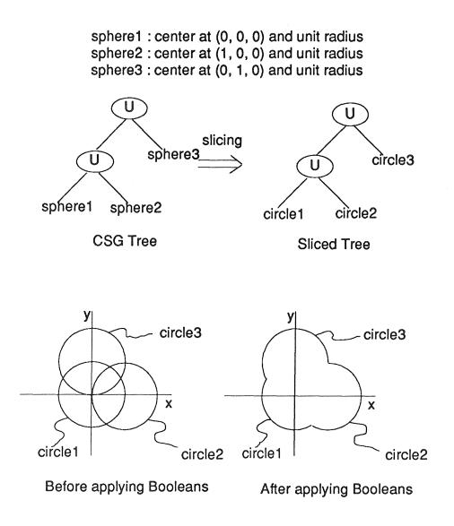
Figure 3. CSG slicing and set operations for SFF [7].
