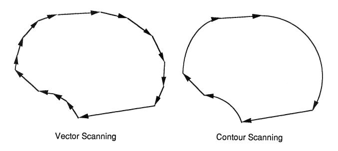
Figure 6. Contour scanning.
