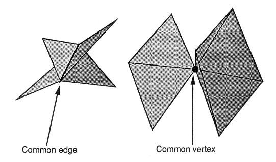
Figure 2. Other examples of non-manifold topology in a faceted SFF model.
