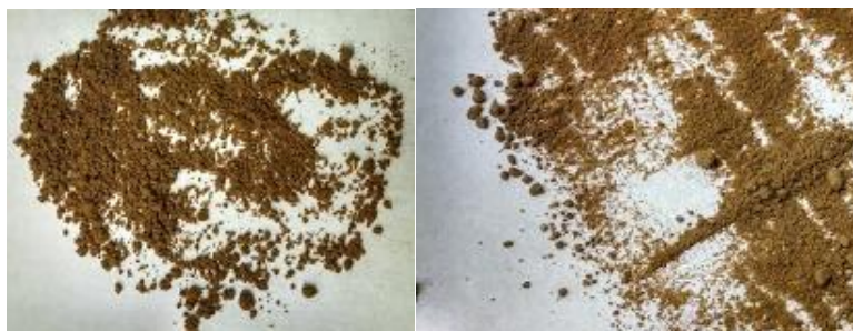
Figure 9.7 - Loose RMA soil, a) 14.5% GWC b) 7.5% GWC
