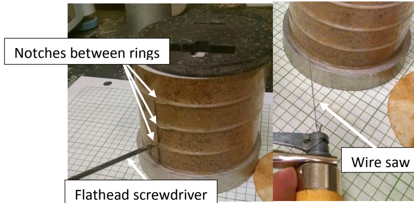
Figure 7.5 - Slicing of centrifuge sample
