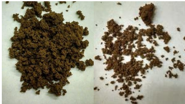
Figure 9.6 - Loose RMA soil, 21.5% GWC
