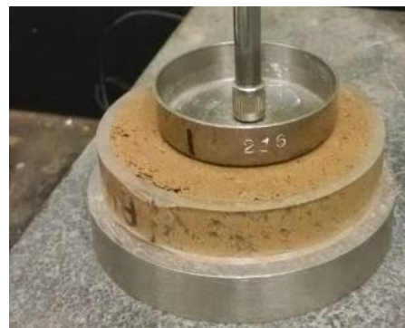
Figure 7.6 - Measurement of slice height
