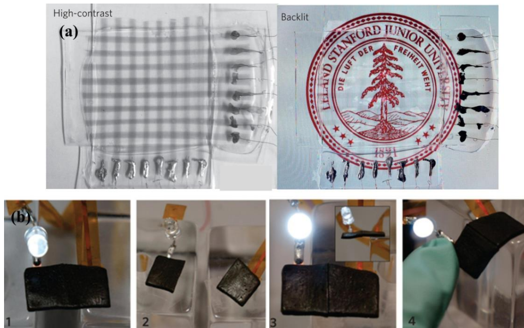
Fig. 1.8 (a) Flexible sensor array based on active-matrix circuitry; (b)Self-healing composite mixed by oligomer chains and \mu Ni particles
