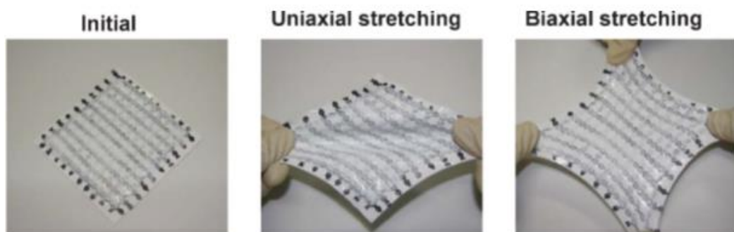
Fig. 1.13 T.Someya's group designed an Ag electrode coated transistor interconnected by elastic conductors on PDMS sheet which can sustain some biaxial stretching
