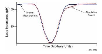
Fig. 8. Car on the edge of the square loop
