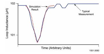
Fig. 9. Car passing over the diamond loop
