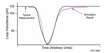
Fig. 10. Car on the edge of the diamond loop
