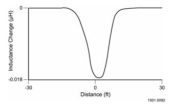
Fig. 18. Motorcycle passing over multiturn loop 2
