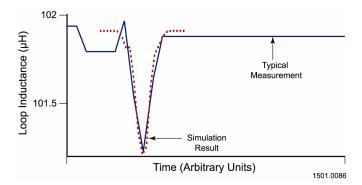
Fig. 12. Motorcycle passing over the diamond loop
