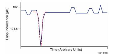
Fig. 13. Truck passing over the square loop
