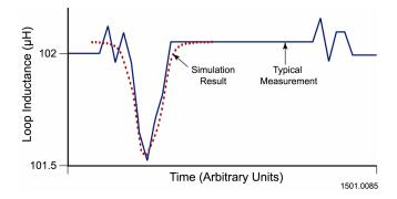
Fig. 11. Motorcycle passing over the square loop
