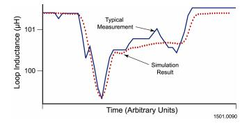
Fig. 16. Car passing over multiturn loop 2
