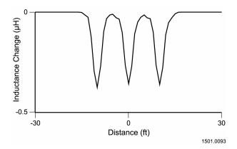
Fig. 19. Truck passing over multiturn loop 2
