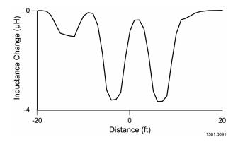
Fig. 17. Car passing on the adjacent lane of multiturn loop 2
