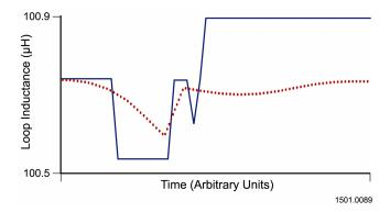
Fig. 15. Truck passing over the diamond loop
