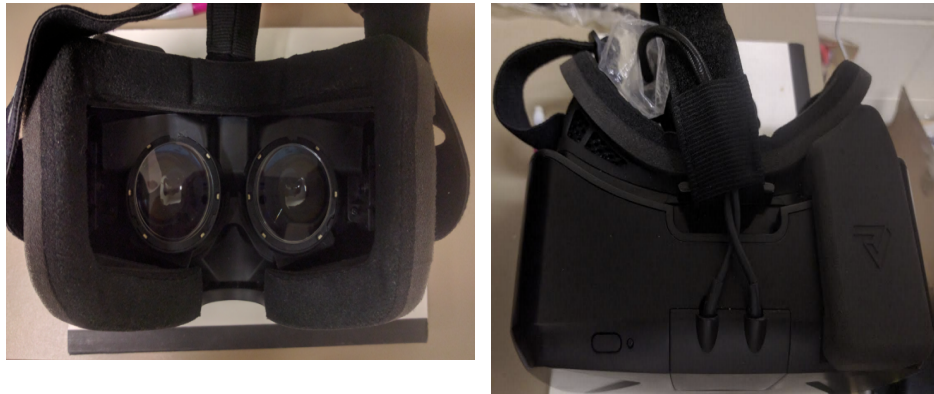
Figure 30: Left: Objective lenses as viewed by the wearer. Right: Top view of the HMD with the eye tracker upgrade
