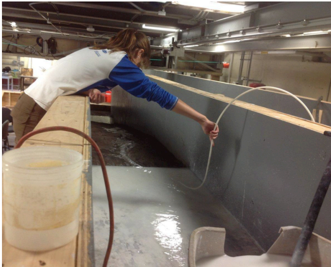
Figure 4.6 Injection of the mix of titanium dioxide and water into the pooled water upstream of the sloped surface. Picture by David Bauer.
