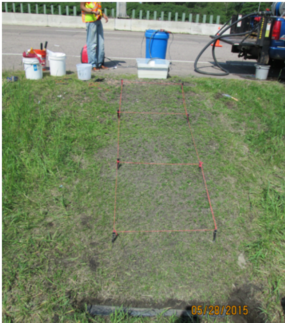
Figure 5.1 Grassed roadside swale at Hwy 77 after cutting and raking the surface vegetation.
