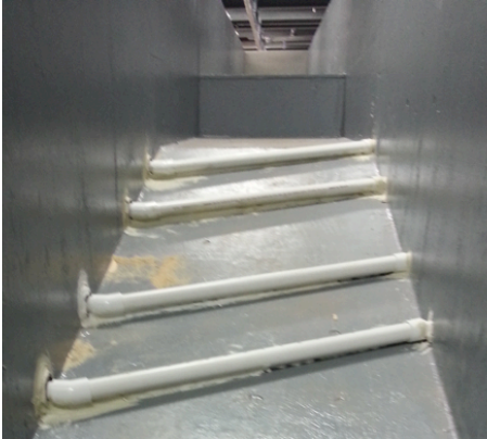
Figure 4.2 Image of four of the perforated drain pipes underneath the soil in the flume.
