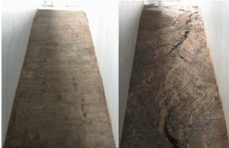
Figure 4.10 Initially smooth surface at t=0 min and after 60 min of simulated runoff.
