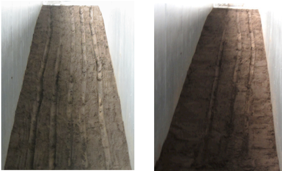
Figure 4.5 Left: Surface with 5 initial rills. Right: Surface with 3 initial rills.
