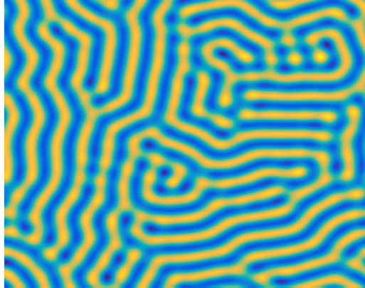
Figure 1.1.1: Evolution of the cubic Swift-Hohenberg equation in two spatial dimensions from small random perturbations of the state u \equiv 0 . Patches of coherent stripes form which interact along various slowly evolving defects.
