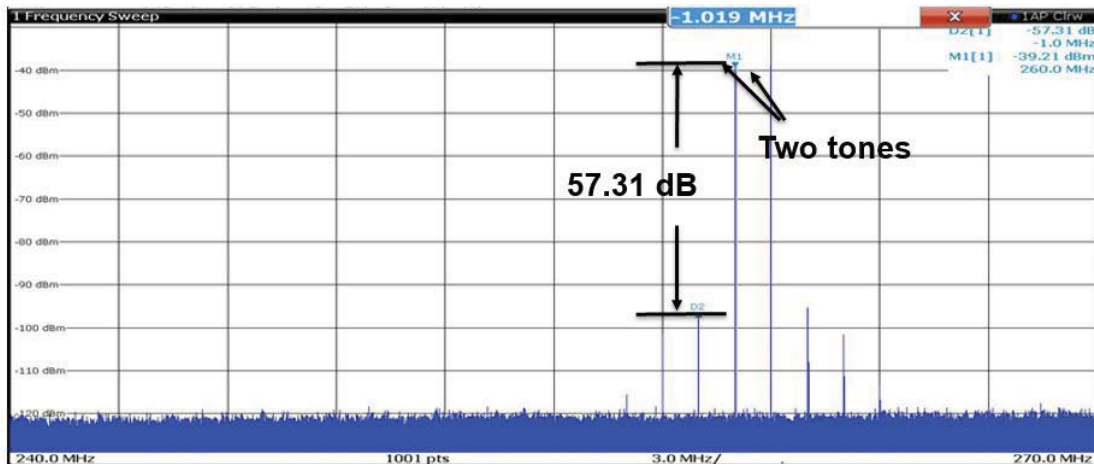
Figure 6.14: Measured IM_3 at 260MHz, V_c = 1.1V , with tones separated by 1MHz
