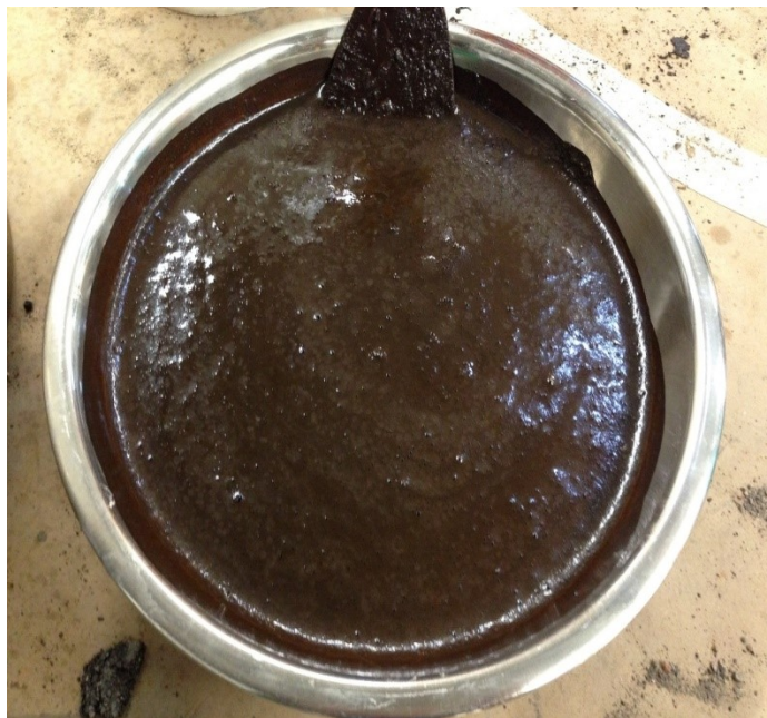
Figure A1: Slurry Trial Mix Immediately after Mixing.
