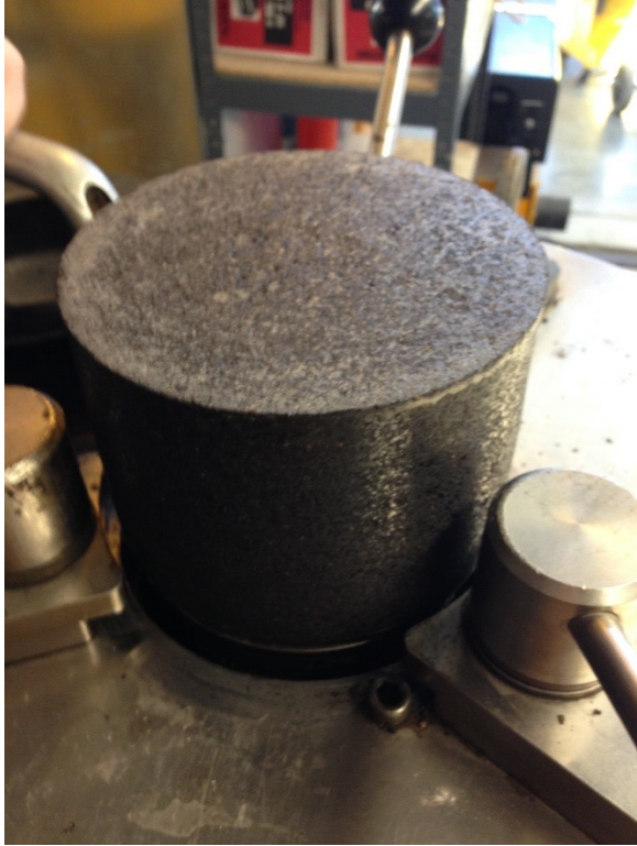
Figure A3: Slurry Trial Mix after Compaction in Gyrotory Compactor.
