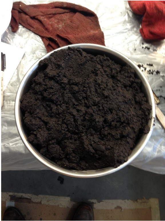
Figure A2: Slurry Trial Mix after Placement in Oven for Two Hours (Curing Simulation).
