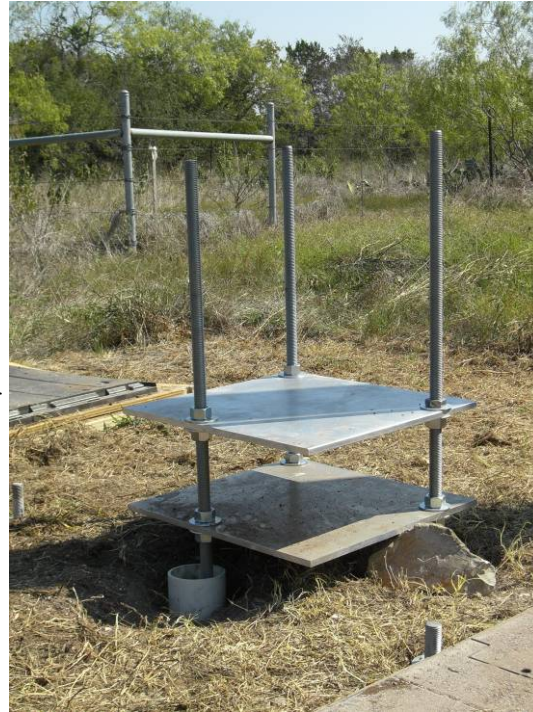
Figure 2.16: Gravimeter monument at site of Green Emerald Terrace. Left panel is the sketch diagram (not to scale). There are three post supporting SG dewar and mounting on one-inch rod, which is cemented into hard rock about 18 inches (45.72 cm). Two \frac{3}{4} inch (1.9 cm) aluminum plates are used to align three pillars. The lower one is used during cementing and the upper one is used during gravimeter installation. Right panel is the picture taken before the floor laid and gravimeter installation. The heights of two plates are adjustable during gravimeter installation.
