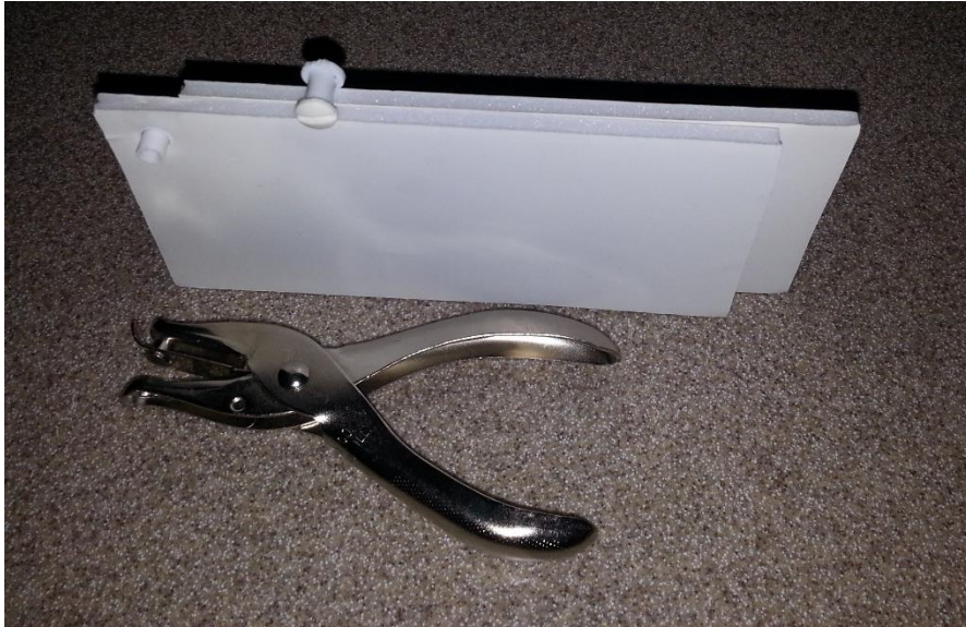
Figure 14: Screw-insert (Detachable Pin), Foam-board, Hole-punch for Four-bar Linkage Physical Prototyping
