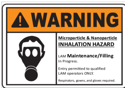
Figure 6. The “Maintenance/Filling” warning sign for display outside the door during LAM maintenance or filling operations. This indicates that some part of the LAM apparatus is open to air.
