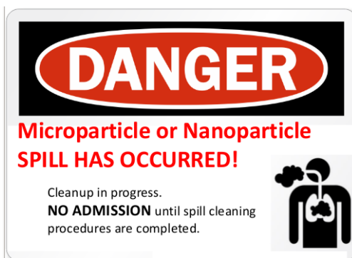
Figure 7. The “Spill” warning sign for display outside the door during emergency situations. This indicates that a microparticle or nanoparticle spill has occurred.
