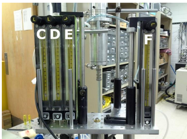
Figure 12. C, D, E, and F – Omega FT-062-01-ST-BN flow controllers.
