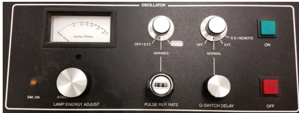
Figure 13. GCR oscillator control panel.
