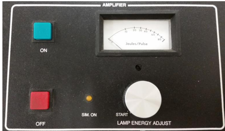
Figure 13. GCR amplifier control panel.
