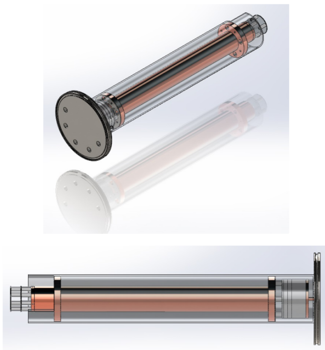
Figure 7.10: A CAD model of our Wiley-McLaren time-of-flight spectrometer [46]
