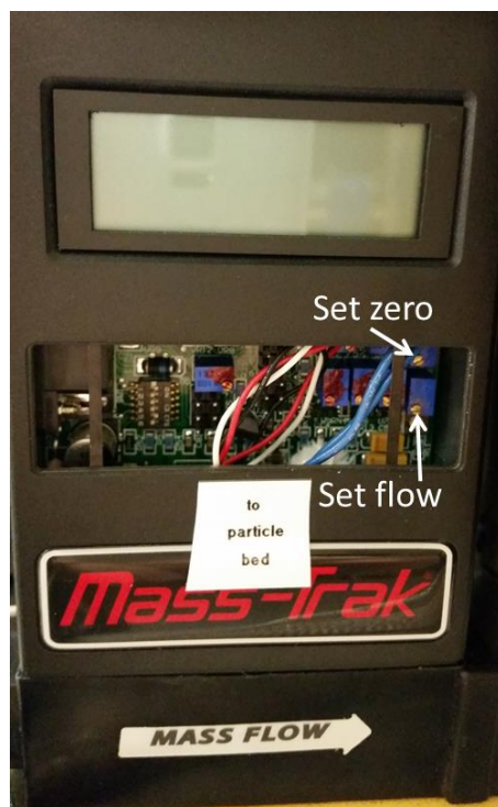
Figure 11. Sierra Instruments, Inc. 810 Mass-Trak Flow Controller. The screws referred to in the Procedure are indicated by arrows and labelled.
