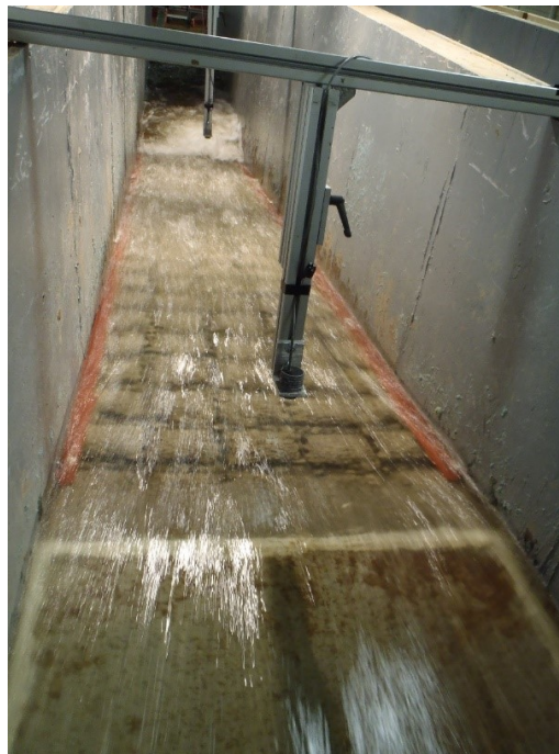
Figure 4.99. View from shoulder looking downstream during 10-12 hour run. No noticeable erosion on the slope.
