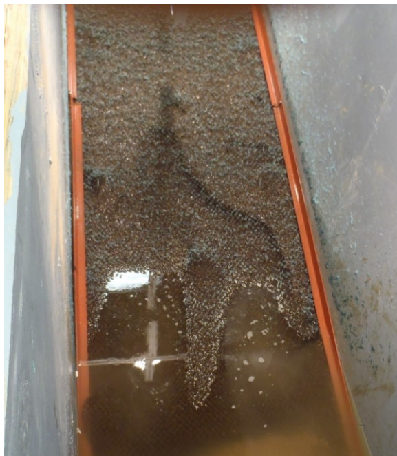
Figure 4.75. View from downstream after 3.5 hours of run time. Erosion working up the slope from the toe under the TRM.
