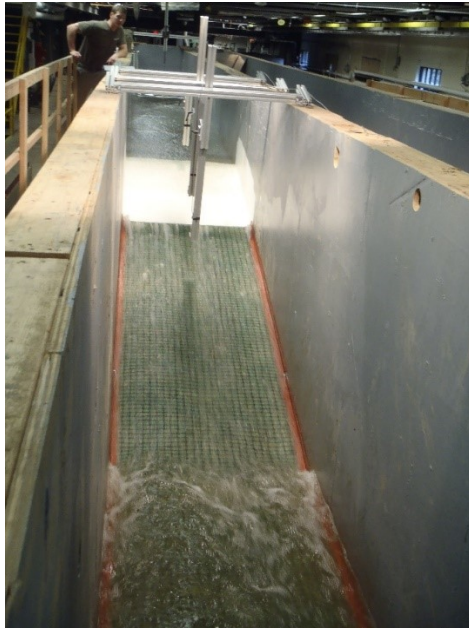
Figure 4.44. Looking upstream at slope with no noticeable erosion. Note the clear tail water.
