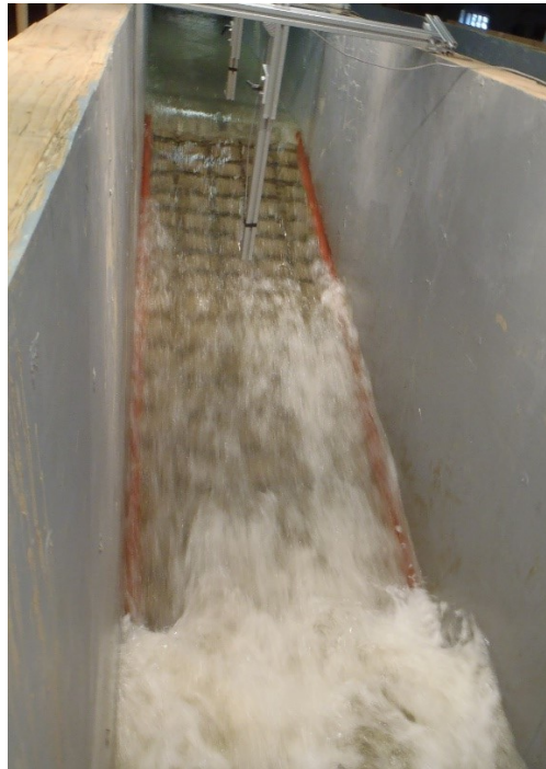
Figure 4.108. View from downstream looking up at slope during 17.25-20.25 hour run. The slope did not drastically change over 10 hours of run time from the first sign of erosion.
