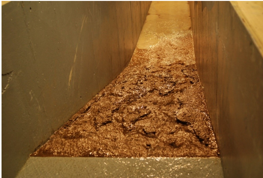
Figure 4.2. 4H:1V Slope mid-run with prevalent channels of flow looking downstream. Less than two minutes of run time.
