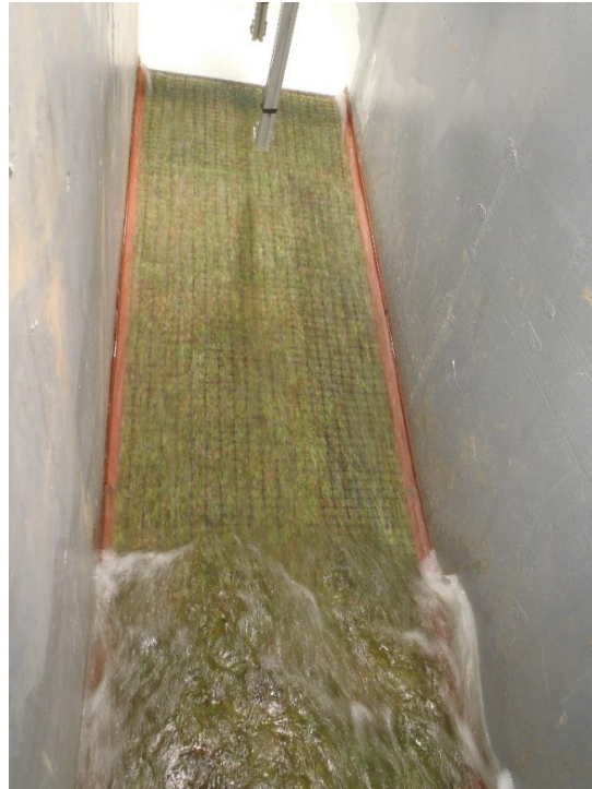
Figure 4.63. Looking upstream during first two hour run, no noticeable erosion anywhere on slope.
