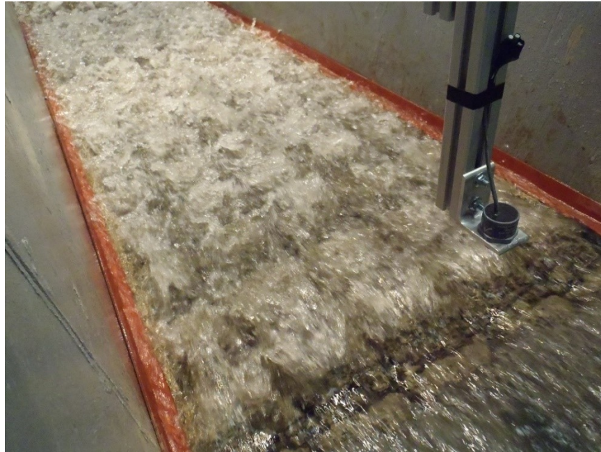
Figure 4.105. View from shoulder looking downstream during first two hour run. Highly turbulent flow but no noticeable erosion on slope.
