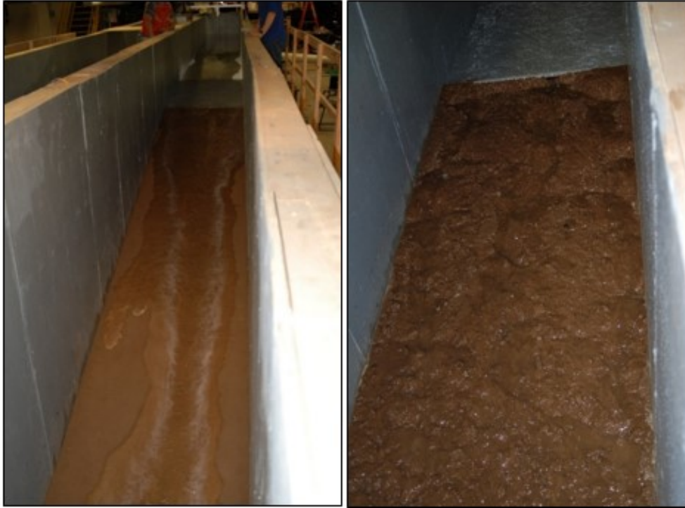
Figure 4.8. (Left) Initiation of flow on 6H:1V slope looking upstream. (Right) Erosion began immediately with incisional channels forming on slope.
