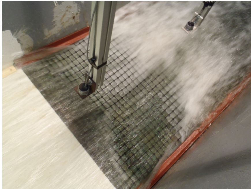
Figure 4.47. Looking downstream from shoulder near the end of the 4-6 hour run. Note the widespread area of erosion and flow separation from the shoulder hitting an angle where the deepest area of erosion is located.
