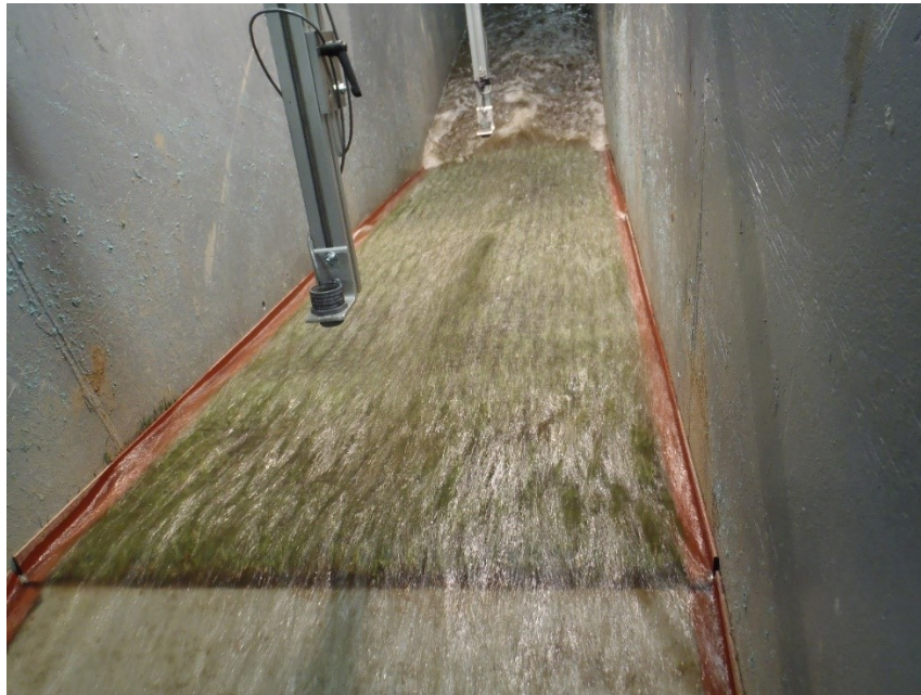
Figure 4.55. Looking downstream from shoulder. Testing 30-60 min, no noticeable large areas of erosion.
