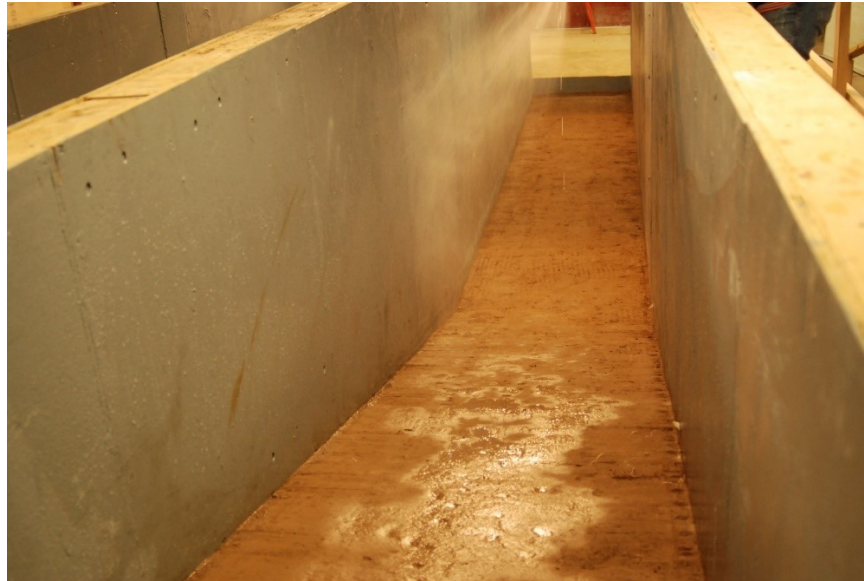
Figure 4.1. Pre-run 4H:1V slope bare soil looking downstream from shoulder.
