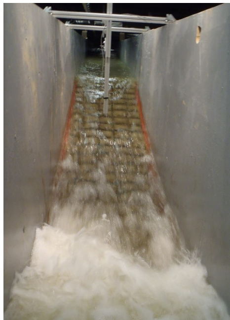
Figure 4.106. View from downstream looking up at slope during 24.35 to 25.33 hour run. Mid-slope mound has been eroded and flat upper slope has stabilized and new mound at toe of slope is causing aeration.
