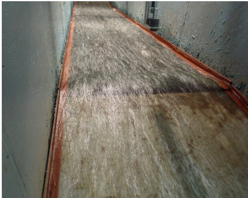
Figure 4.83. View from upstream during 2-4 hour run. Noticeable depression after shoulder along right edge of slope. More of the FRM is being removed from testing.
