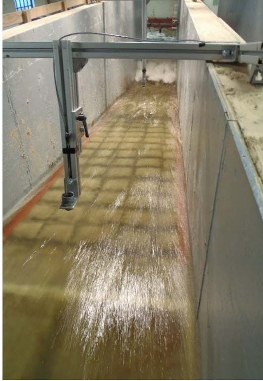
Figure 4.100. View from shoulder looking downstream during 22-24 hour run. No noticeable erosion, smooth water surface to about mid-slope.
