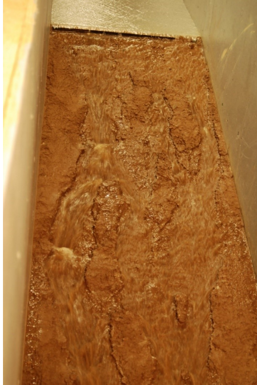
Figure 4.3. Mid-run 4H:1V slope looking upstream. Flow channelized on slope with trough forming on the transition from shoulder to slope.
