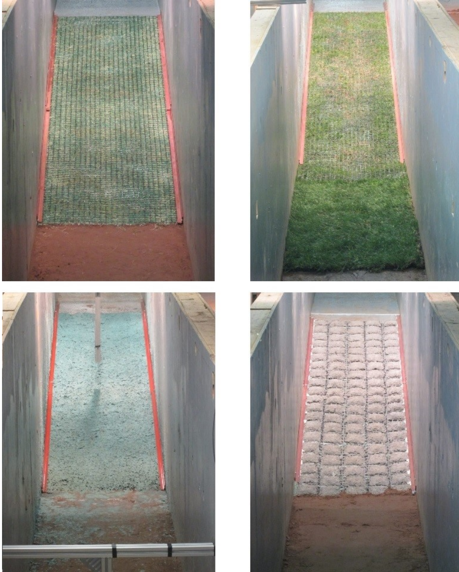
Figure 3.9. Stabilization techniques tested. Upper left: Technique 1, “Armored Sod” with erosion control blanket; Upper right: Technique 1A, “Armored Sod” with real sod; Lower left: Technique 2, Turf Reinforcement Mat (TRM) with Fiber Reinforced Matrix (FRM); Lower right: Technique 3, Flexible Concrete Geogrid Mat.
