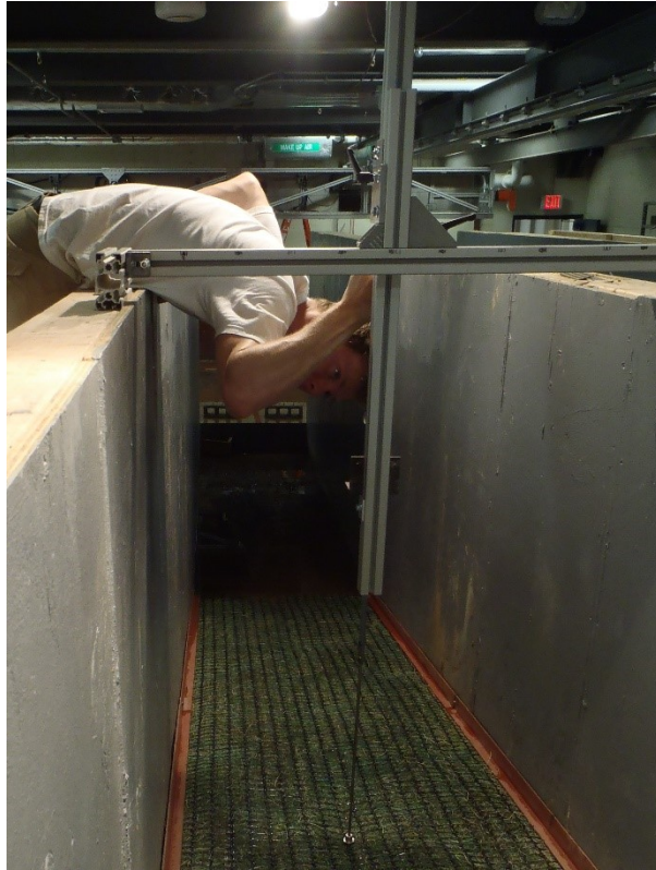
Figure 3.20. Point gauge being used on slope to check for erosion and voids in soil beneath erosion control blanket.
