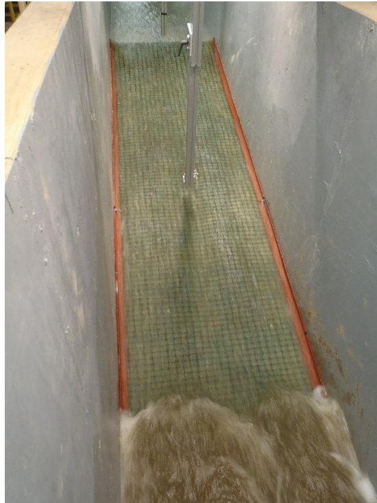
Figure 4.20. Looking upstream at slope no erosion occurring at 1.1cfs.
