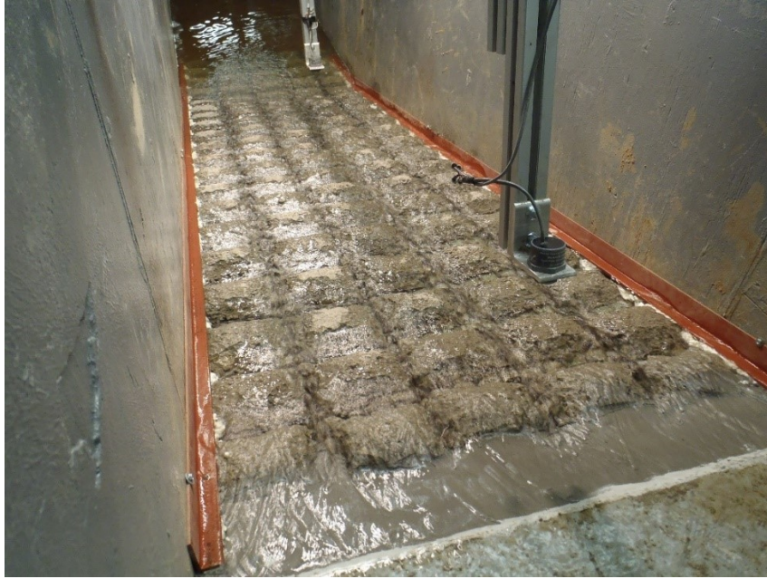
Figure 4.91. Image from Run 1 with discharge set at 0.9 \text{ ft}^3/\text{s} . There was no noticeable erosion over entire 30 min run.
