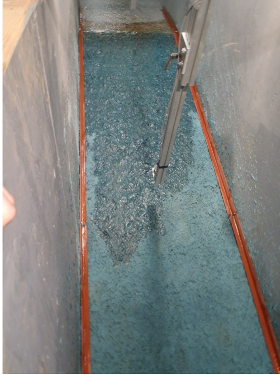
Figure 4.72. First run on TRM-FRM at 0.89 cfs and 0.5-inches of overtopping.
