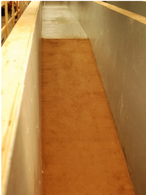
Figure 3.6. Prepared bare soil slope in the flume.
