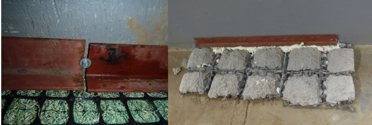
Figure 3.18. Angle iron fastened to flume wall (left). Flexible concrete geogrid mat installation example with backer rod and spray foam insulation used to fill the void between the Flexamat ® and angle iron resting on top of concrete (right).
