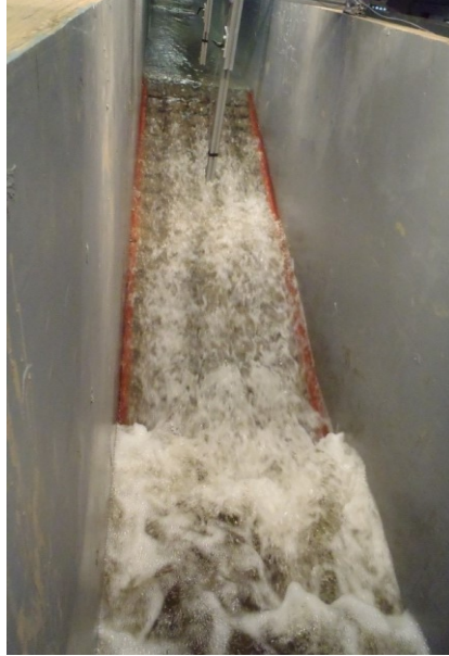
Figure 4.107. View from downstream looking up at slope during 4-6 hour run. Note the depression and subsequent aggradation at mid-slope causing aeration.
