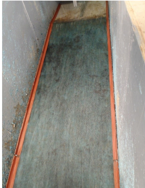
Figure 4.82. View from downstream during 0-2 hour run. Minimal erosion noticed. FRM is being washed away while TRM is remaining stapled to the slope.
