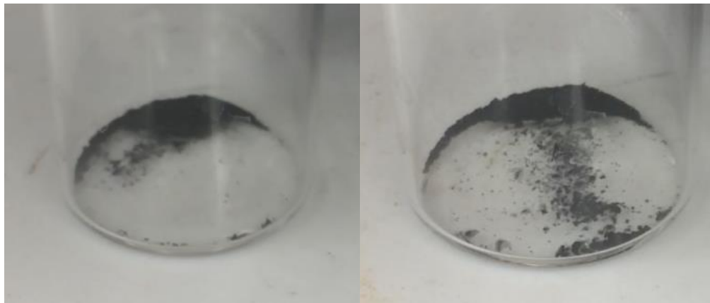
Figure 6. Movement of Fe 3 O 4 -TiO 2 -CNTs on stir plate. Left: Initial. Right: After brief stir
