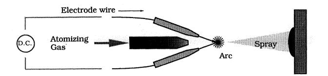
Figure 2: Schematic of Arc-Spray System.
