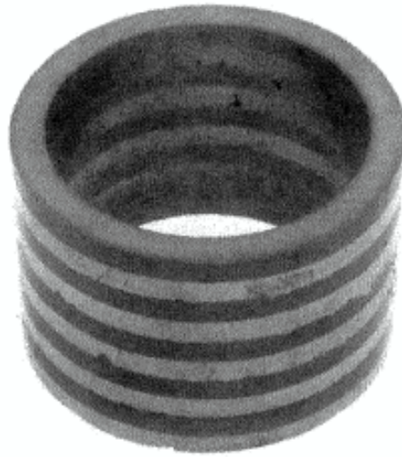
Figure 6. Layered copper steel tube manufactured in MD*
