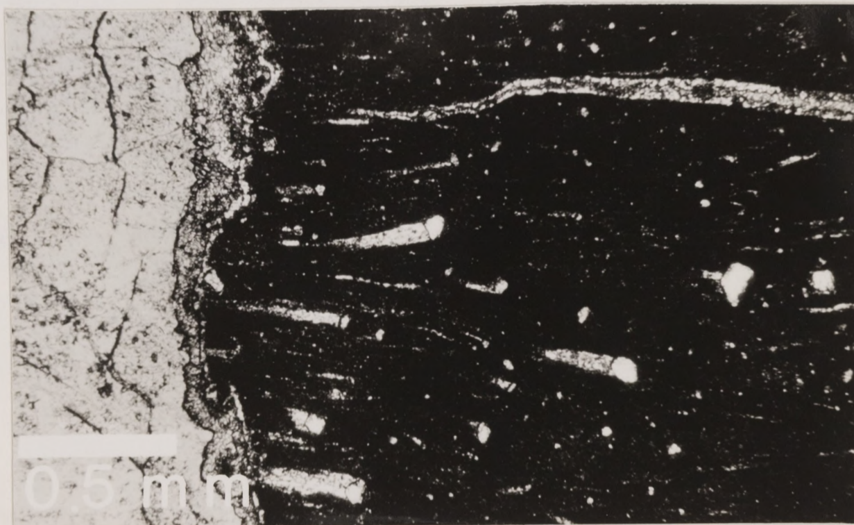
Figure 19. Exterior margin of pisolitic nodules with dark area that contains abundant ferric oxide, clay minerals, and quartz silt in microspar matrix. Toward interior (left) is dolomite and sparry calcite filled fracture.
