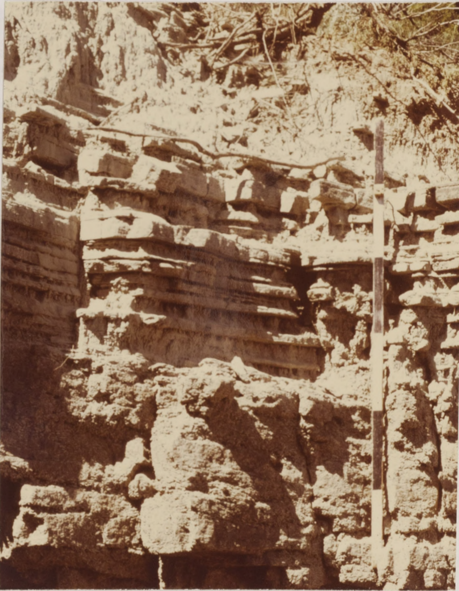
Figure 24. Fining upward delta front deposits exposed at DD-6b. Staff is 1.8 m (6 ft).
