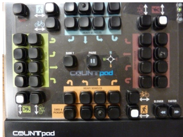
Figure 10: Electronic Count Board Used With Video Data Processing
