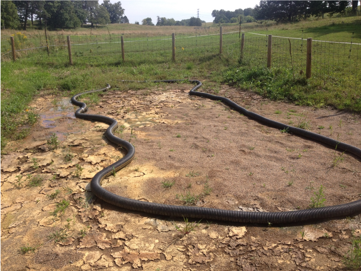
Figure 30. Iron Enhanced Sand Filter when maintenance is needed. (Note: the black perforated tile line on the surface of the IESF was used to distribute flow evenly across the surface, though it was unsuccessful because it became clogged with iron ochre. It was subsequently removed shortly after this picture was taken).
