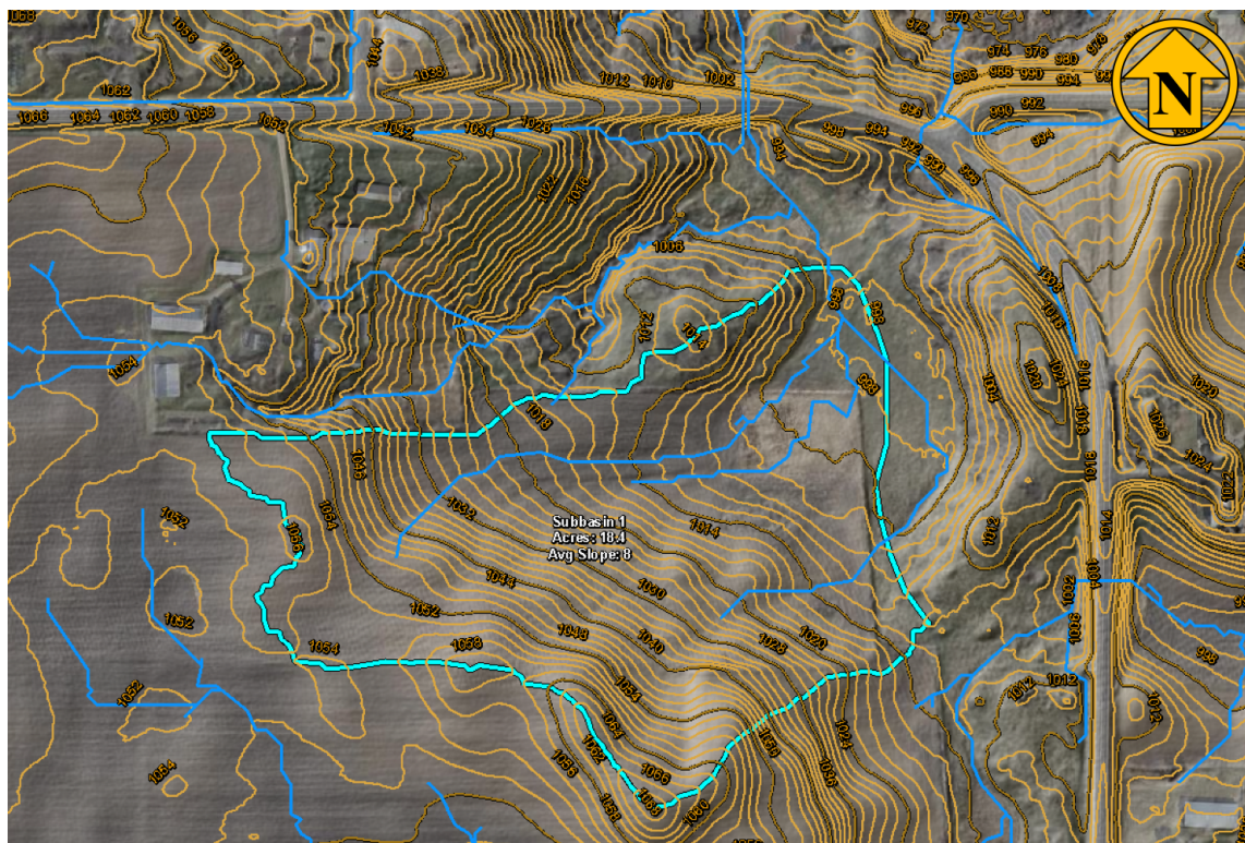
Figure 3. Surface contours (orange lines) around iron enhanced sand filter (IESF) location. Subwatershed draining to IESF shown in light blue, approximate location of surface channels shown in blue (courtesy Minnesota Department of Agriculture).
