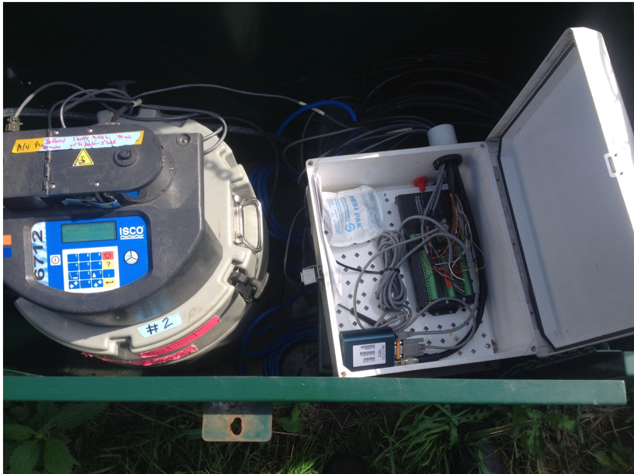
Figure 36. Monitoring: ISCO 6712 automatic water sampler (left), Campbell Scientific CR1000 datalogger (top right inside white box), and Raven XT cellular data modem (bottom left inside white box).
