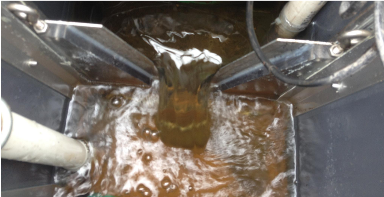
Figure 7. Custom V-notch weir with upstream and downstream pressure sensors (inside white PVC pipes).
