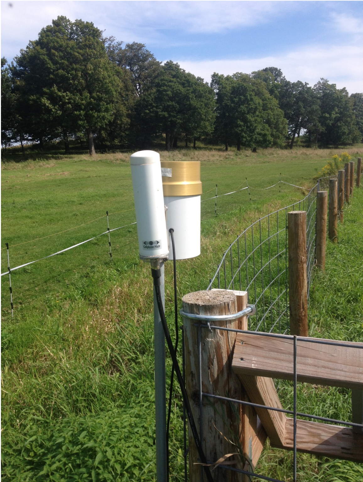
Figure 37. Monitoring: Texas Instruments rain gauge (white cylinder with gold lid) and cellular antenna (white cylinder).
