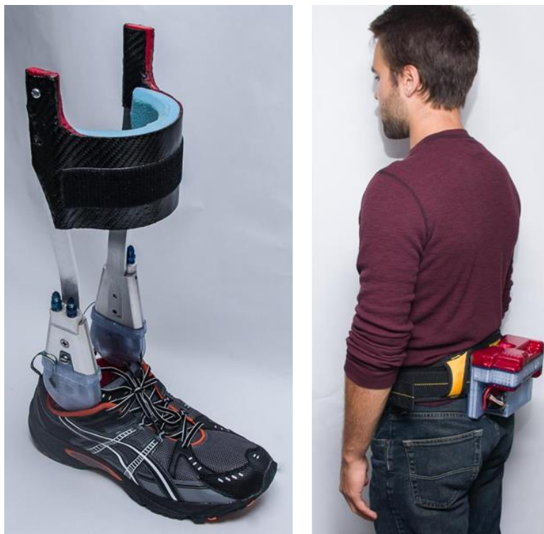
Figure 6.15 Prototype ankle foot actuator (left) and power supply positioning on a user (right)
