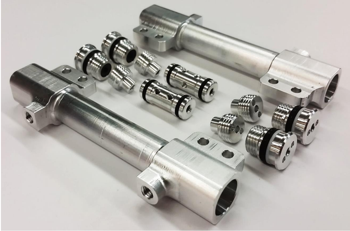
Figure 7.10 Prototype miniature piston cable hydraulic cylinders
