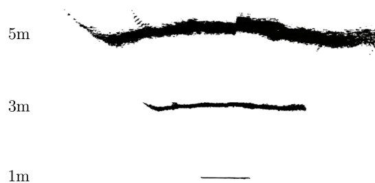
Figure 3.9: Raw data from a PrimeSense Carmine device of a flat wall at varying distances. Reproduced from [66].
