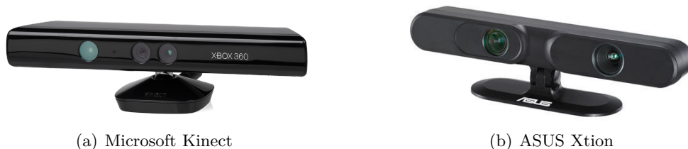
Figure 3.3: Example RGB-D sensor, based on the PrimeSense Carmine reference device. ASUS Xtion image taken from ASUS webpage: https://www.asus.com/3D-Sensor/Xtion_PRO/
