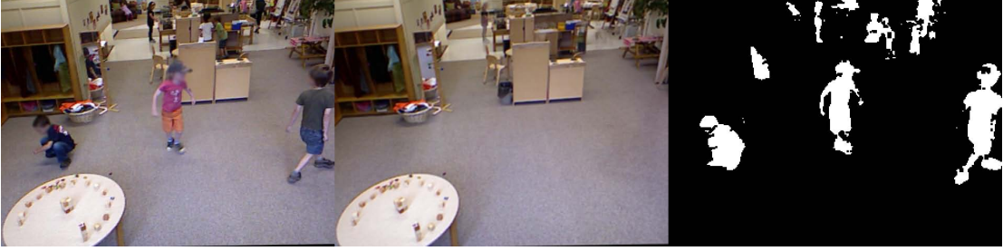
Figure 3.12: Sample frame demonstrating the robust PCA background subtraction step, splitting an input test frame (left) into the background model (middle) and foreground error. The foreground error is thresholded to yield a binary foreground mask (right).
