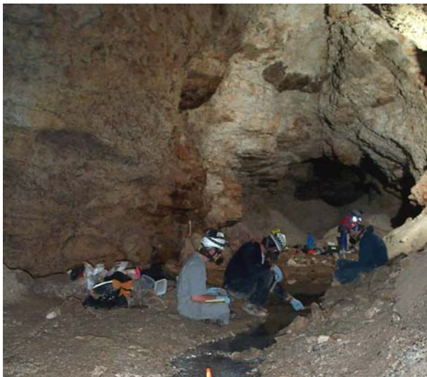
Figure 4.3: Performing a salt dilution trace at the outflow channel just downstream of the Upper Spring orifice. Note the linear fracture running through the ceiling in the upper right side of the picture. The thick bacterial mats start at roughly the location of the yellow stake visible in the bottom of the picture. The gas masks are worn for protection from any organic sulfur gases and the high levels of radon gas. Photo courtesy of A. Engel, 2001.
