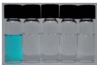
Fig. 6 Colorimetric response of SQ at 14.0 \mu M upon the addition of 2.2 equivalents of various agents in the solution of 1 (0.2 mM) in methanol containing 3.0 equivalents of K_2CO_3 : from left to right (a) CEES (b) CEEE (c) DCP (d) DFP (e) DECP.
