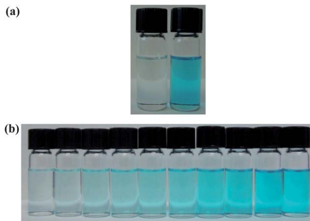
Fig. 4 (a) Colorimetric response of SQ in CHCl 3 at 14.0 μM, from left to right: SQ + 1 in MeOH (51 μM), SQ + [ 1 (51 μM + CEES (112 μM))]. (b) Colorimetric response of SQ with subsequent addition of CEES (from 11–110 μM) from left to right.
