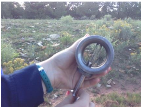
Figure B-4. Fox #FT3 velocity probe centered in a 2” nominal diameter stack.
