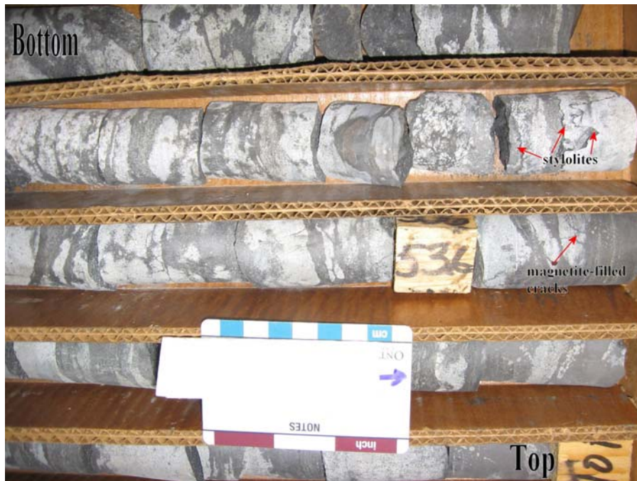
Figure 19. Photograph of drill core displaying the various bedding types present in the Variably-Bedded and/or Mottled Unit of the Lower Cherty (LC-5A submember at Minntac). Note the highly irregular nature of the dark-colored magnetite-rich bands and zones. Note also the magnetite-filled “cracks” across clasts (no transport indicated) and the magnetite-filled stylolites (upper right). Drill hole #24426 from 532 feet through 540 feet.
