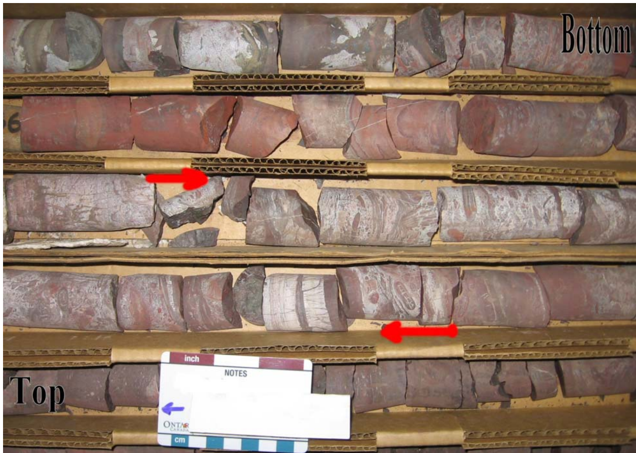
Figure 35. Photograph of drill core displaying the various textures and bedding types associated with the Algal Unit at Minntac (UC-15 equivalent). Oncolites, some with syneresis cracks, are present between the red arrows. Drill hole #24426 at 264-278 foot depth.
