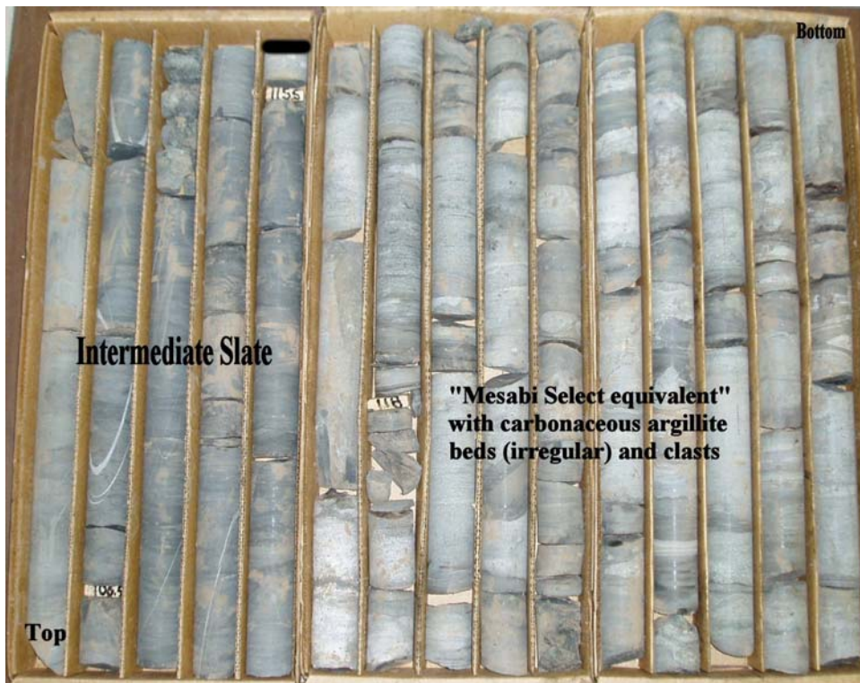
Figure 29. Photograph of drill core displaying the potpourri of rock types constituting the Lowermost Thin-Bedded Unit of the Lower Slaty at the East Reserve/McKinley Extension mine near Biwabik, MN. Drill hole #15-15 from 104.5 feet to 135 feet. Note the thick section of black-colored, carbonaceous mudstone (aka the Intermediate Slate Unit) in the left side of photo (104.5-115.5 feet). Core in each row of the boxes = 2 feet long.
