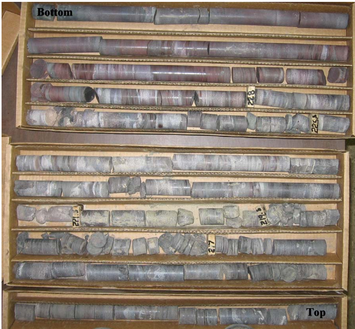
Figure 13. Photograph of thin-bedded rocks of the Basal Red Unit in drill core at the East Reserve/McKinley Extension (LC2 submember); drill hole 31-7, 212-235 feet. Note that a red color is dominant only at depth (227-235 feet) in this hole. Core in each row of the boxes = 2 feet long.
