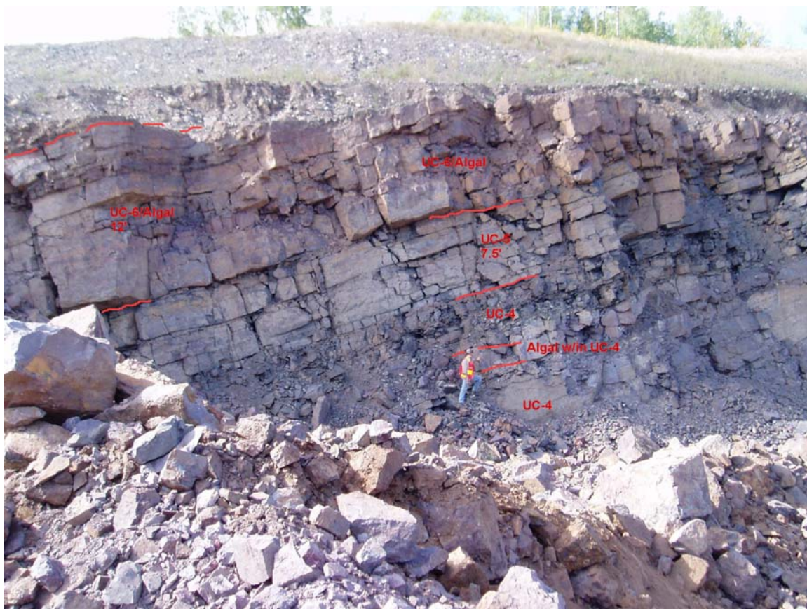
Figure 36. Photograph of geologic units associated with the top of the Lower Slaty and bottom of the Upper Cherty at the Laurentian mine. Note the presence of two algal horizons. One is positioned near the base of the Upper Cherty (UC-6 submember in the photo; approximately twelve feet thick), and the other (two feet thick within the UC-4 submember of the photo) is positioned near the top of the Lower Slaty. The UC-submember nomenclatures on this photograph are Utac designations, and these designations were applied during mapping of the pit by NRRI geologists. Conversely, the entire bench, as depicted in the photograph, is considered to be within the ArcelorMittal’s UC-3 submember (see Fig. 34).
