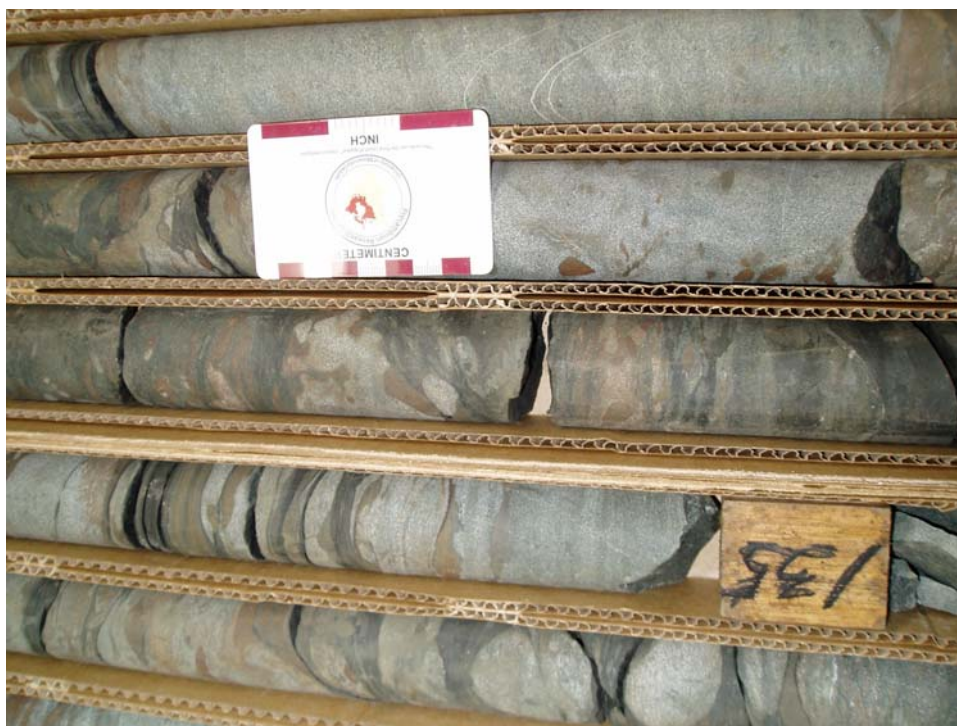
Figure 30. Photograph of drill core displaying the potpourri of rock types constituting the Lowermost Thin-Bedded Unit of Lower Slaty at the East Reserve/McKinley Extension mine near Biwabik, MN. Jones and Laughlin drill hole #6549 at 134 feet to 141 feet.
