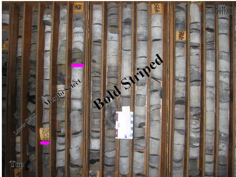
Figure 22. Photograph of drill core displaying typical Mesabi Select (480-485.5 feet) and Bold Striped (485.5-502 feet) units associated with the LC-5B submember at Minntac. Also shown are thin-bedded rocks of the Lower Slaty member (mostly dark-colored rock at 476-480 feet). Drill hole #24426 from 476 feet to 502 feet. Core in each row of the boxes = 2 feet long.
