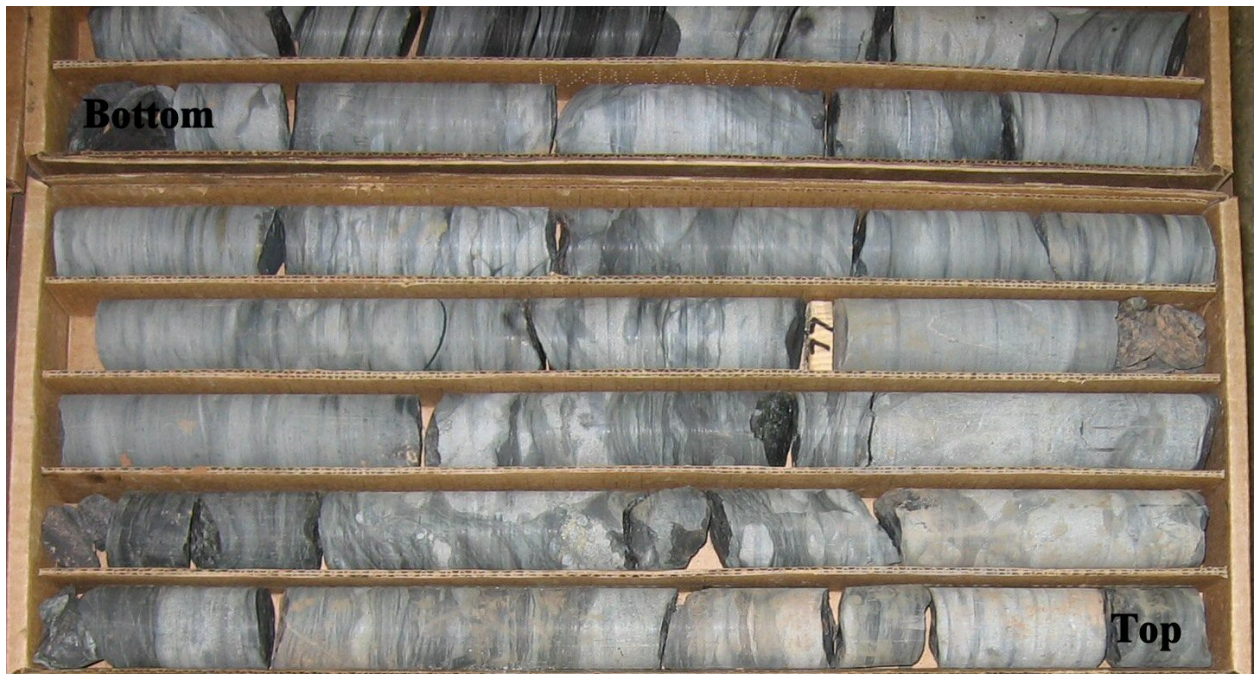
Figure 32. Photograph of drill core displaying scrambled-bedded and flowage of the black carbonaceous argillite around blocks of “Mesabi Select equivalent” at the East Reserve/McKinley Extension mine. Drill hole #39-7 from 61 feet to 84 feet. Core in each row of the boxes = 2 feet long.
