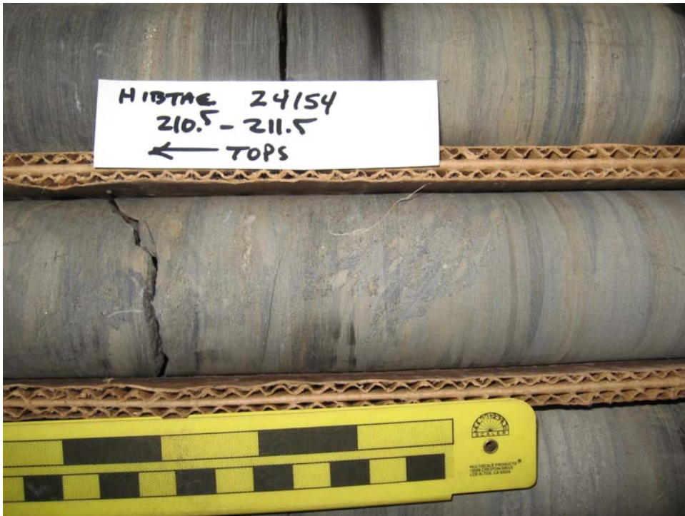
Figure 28. Photograph of drill core illustrating the generation of iron carbonate granules in the Lowermost Thin-Bedded Unit of the Lower Slaty at Hibtac. Drill hole #24154 at 211 feet to 211.5 feet.
