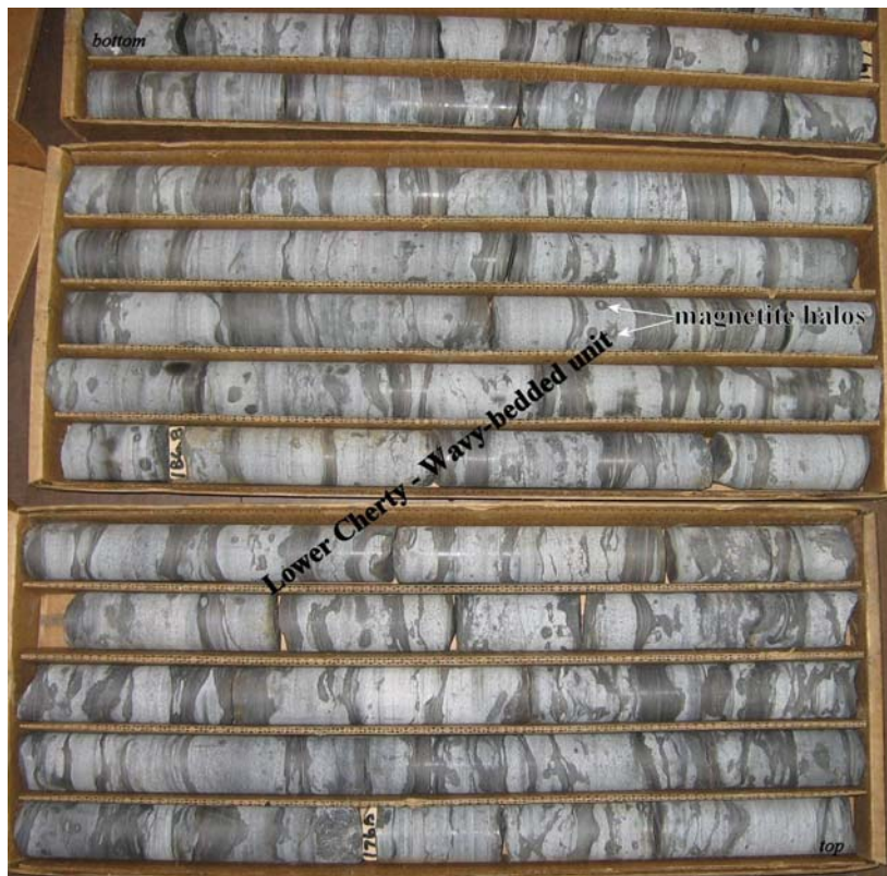
Figure 15. Photograph of drill core displaying typical bedding textures associated with the Wavy-Bedded Unit of the Lower Cherty. Note the pinch-and-swell thickness variations of the dark-colored, magnetite-rich wavy bands, as well as the round magnetite halos around light-colored intraclasts. Photograph of drill core from ArcelorMittal’s LC-4 submember in hole 39-7 at the East Reserve/McKinley Extension (175-199 feet). Core in each row of the boxes = 2 feet long.
