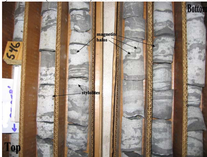
Figure 16. Close-up photograph of drill core displaying typical textures associated with the Wavy-Bedded Unit of the Lower Cherty (LC-4 submember at Minntac). Note nature of wavy magnetite-rich beds (dark), chert bands with diffuse magnetite (moderate gray), occasional magnetite-rich stylolites at contacts (center-left), and magnetite halos (dark ovoids) around cherty intraclasts. Drill hole #24426 from 546 feet through to 556 feet.
