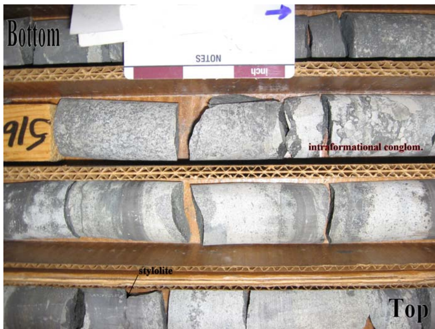
Figure 20. Photograph of drill core displaying typical intraformational conglomerate associated with the Variably-Bedded and/or Mottled Unit of the Lower Cherty (LC-5A submember at Minntac). Drill hole #24426 (from 510 feet through 518 feet) with highly irregular magnetite-rich beds and stylolites.
