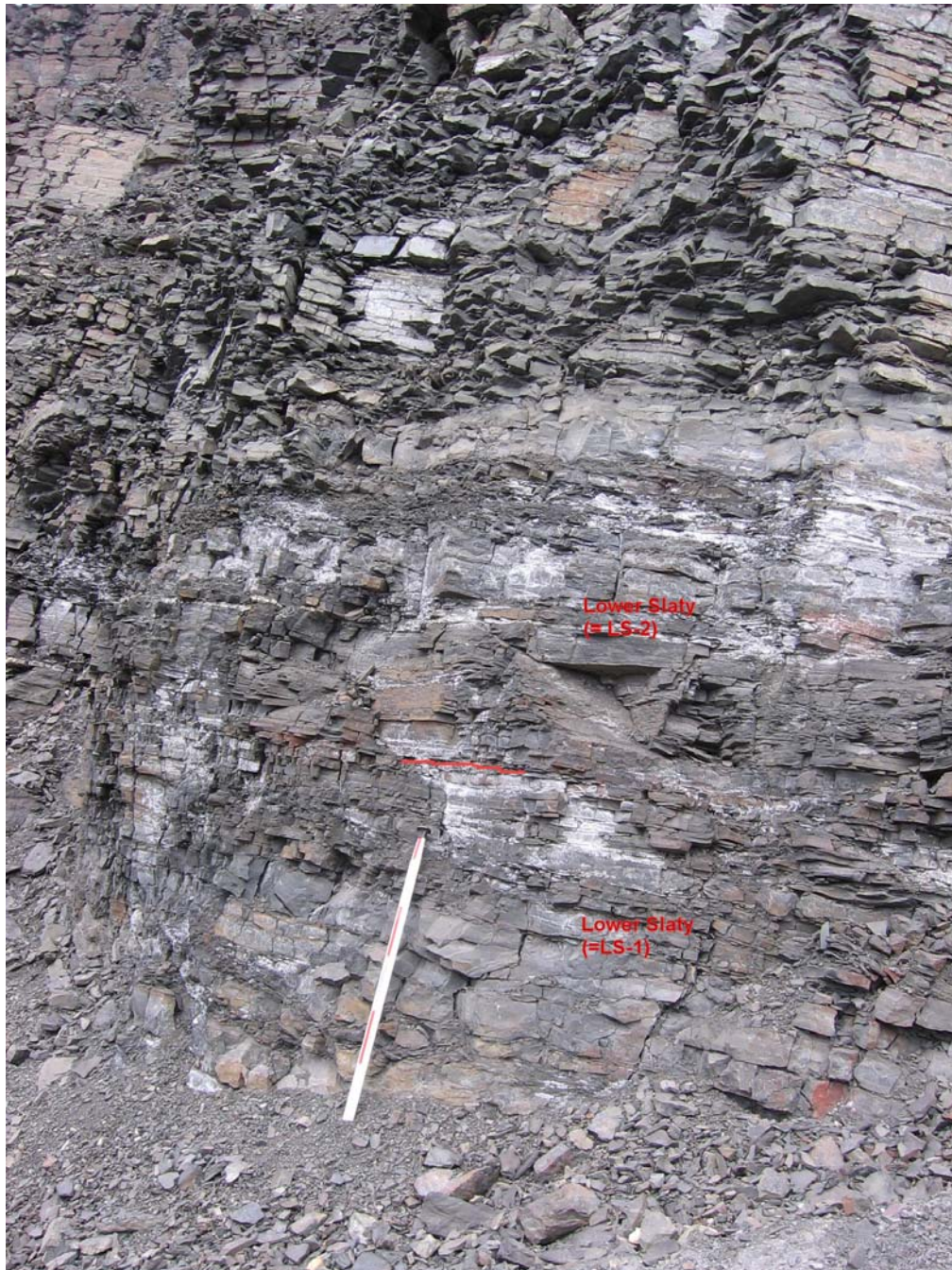
Figure 24. Photograph of a mined bench in the Laurentian Mine displaying the thin-bedded nature of the Lower Slaty member. Stadia rod is marked in one foot increments (alternating red and white bars) and is 5.5 feet long. The Intermediate Slate is present at the base of the bench (the LS-1 submember in the photograph); note the common white coating of melanterite, which is an iron sulfate derived from weathering of sulfides in the iron-formation on the subvertical joint faces. The top part of the bench is characterized by thin-bedded, non-magnetic to weakly magnetic, iron carbonate iron-formation that is characteristic of the Lowermost Thin-Bedded Unit of the Lower Slaty member (the LS-2 submember in the photograph).
