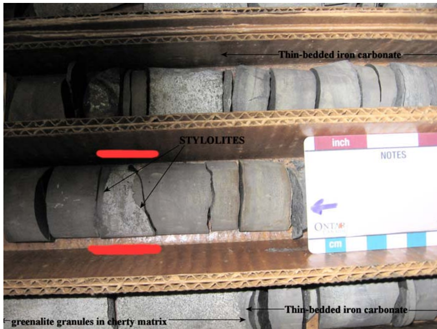
Figure 23. Photograph of drill core displaying carbon-coated stylolite at the contact between a brown-colored iron carbonate bed and a light-colored chert band with greenalite granules. Features shown are typically seen in the Bold Striped Unit of the LC-5B submember at Minntac. Drill hole #24426 at around the 492 foot depth.
