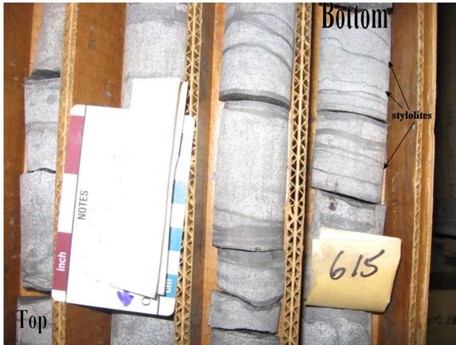
Figure 17. Close-up photograph of drill core displaying typical textures of the Wavy-Bedded Unit of the Lower Cherty member at Minntac (where it is named the LC-3 submember). Note the thin, magnetite-rich, wispy wavy-beds, magnetite-rich stylolites, and salt-and-pepper texture (S&P) due to disseminated magnetite. Drill hole #24426 around 615 feet deep.
