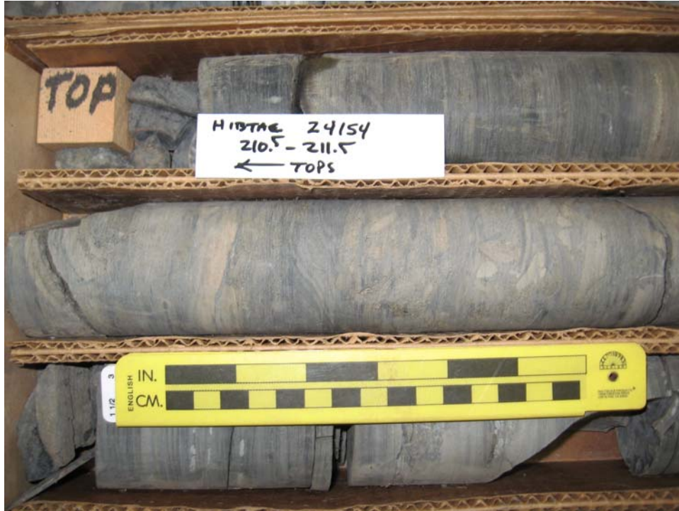
Figure 27. Photograph of drill core displaying disrupted bedding and generation of iron carbonate intraclasts in the Lowermost Thin-Bedded Unit of the Lower Slaty at Hibtac. Drill hole #24154 at 210.5 feet to 211 feet.
