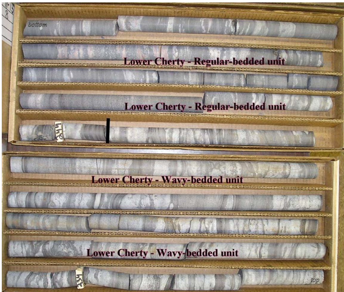
Figure 14. Photograph of drill core exhibiting the bedding characteristics of the Regular-Bedded Unit that exhibits a transitional contact with overlying weakly wavy-bedded rocks. Core shown is from the bottom portion of the Lower Cherty in drill hole 11-15 at the East Reserve/McKinley Extension. Submembers, as defined by ArcelorMittal, are the LC-3 submember (regular-bedded at 248.5-257+ feet) and LC-4 submember (wavy-bedded at +232-248.5 feet). Core in each row of the boxes = 2 feet long.
