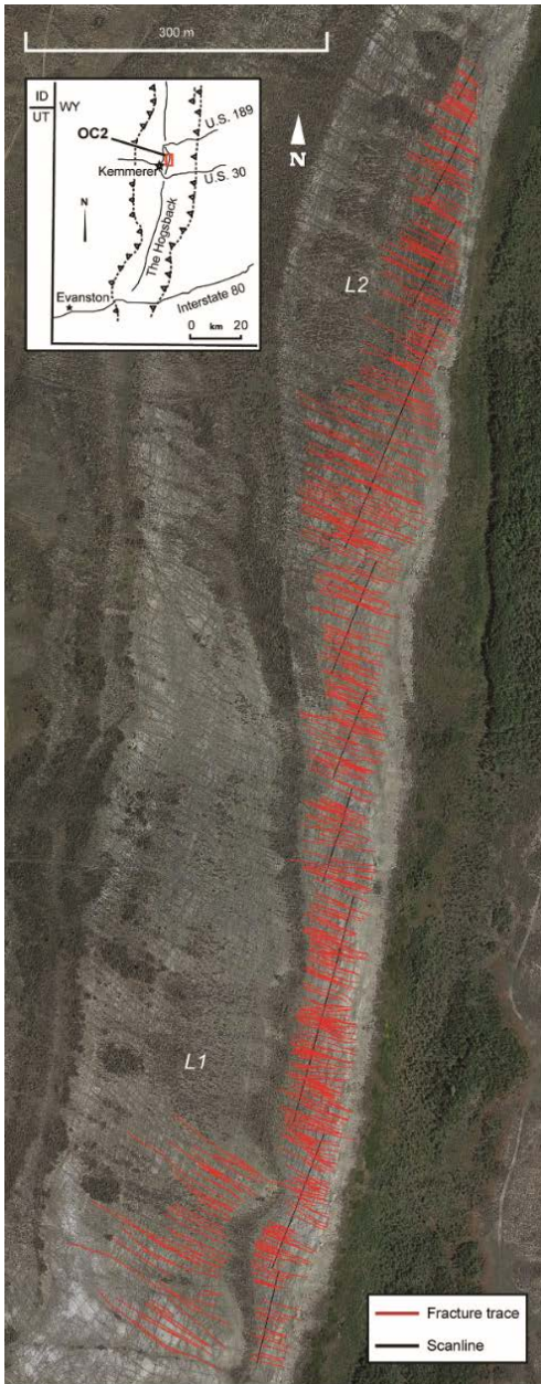
Figure 2-3 Fracture traces, western Green River Basin, outcrop 2 (Oc2 in Figure 2-1). Background Google Earth image where fractures were traced. Red lines mark fracture traces, black lines represent scanlines. Location map after Lorenz and Laubach (1994). Fracture clusters (called swarms; Laubach, 1992, their Figures 4 and 9) are visible in other outcrops on the opposite, steeply east-dipping fold limb.
