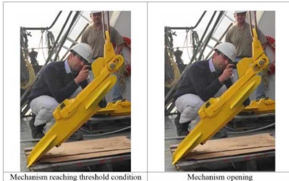
Figure 2.36. Flying Wing Anchor® in Field Test (Jose Eugenio Iturriaga Flores, 2016)
