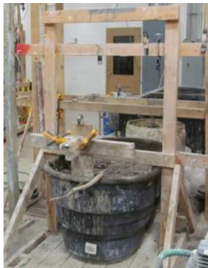
Figure 3.3. Thermoplastic Tank for Preparing Soil Tests Beds
