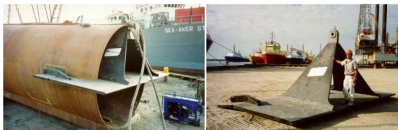
Figure 2.14. Suction Embedded Plate Anchor ( http://www.energetics.com )
