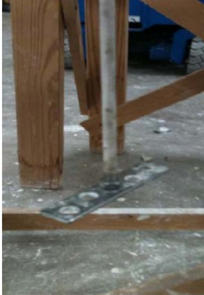
Figure 4.11. Steel Plate Attached to Threaded Rod (Ganjoo, 2010)
