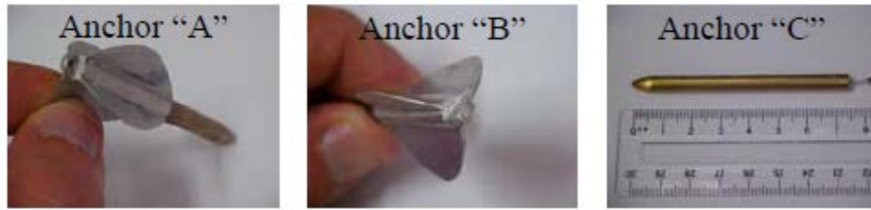
Figure 2.32. 1:200 Scale DPA (O’Loughlin et al., 2004b)
