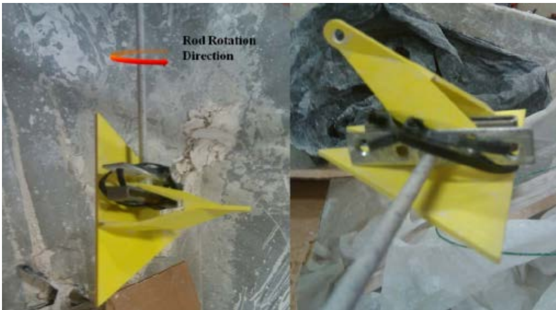
Figure 4.11. Steel Plate Attached to Threaded Rod (Ganjoo, 2010)
