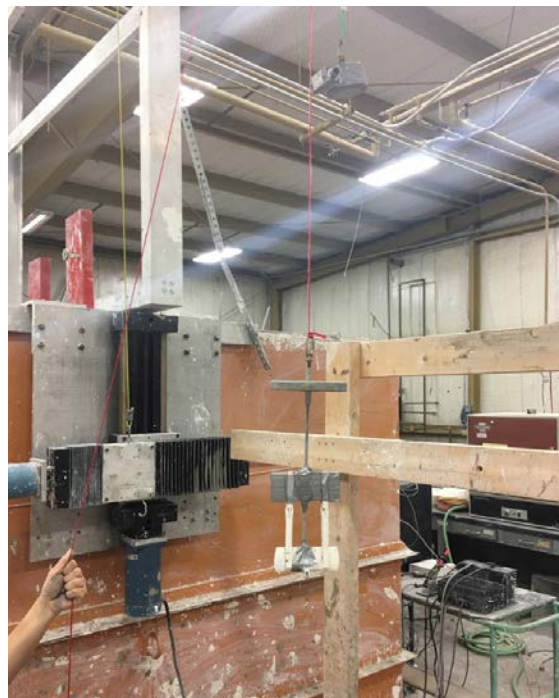
Figure 7.15. Flying Wing Anchor® for Free-Fall Penetration Tests
