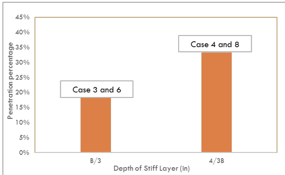
Figure 5.54. Percentage of Tests in Which Stiff Layer Was Penetrated Versus Depth of Stiff Layer
