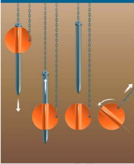
Figure 1.4. Example of Dynamically Embedded Plate Anchor (Blake et al., 2015)
