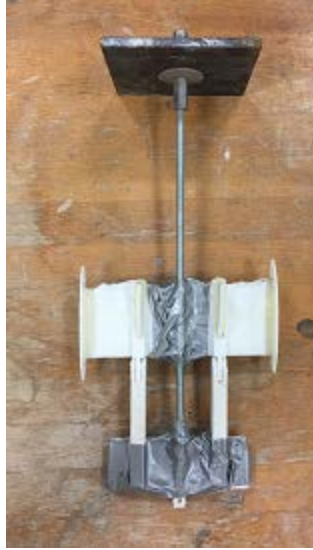
Figure 7.15. Flying Wing Anchor® for Free-Fall Penetration Tests
