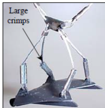
Figure 2.26. Scaled Vryhof Stevmanta (Elkhatib et al., 2002)
