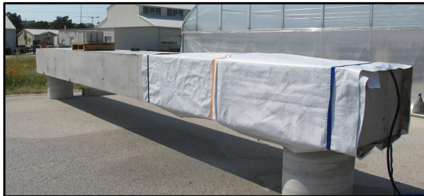
Figure 3-4: Wet conditioning of Zone C
