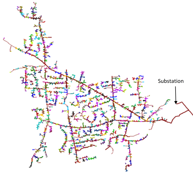
Figure 3.23: One line diagram of the residential distribution circuit (Courtesy of the electric utilities).
