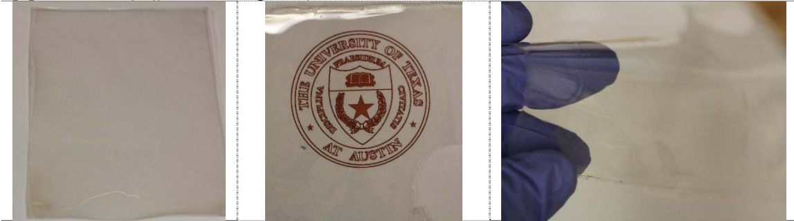
[b] BPS-20K ( \bar{M}_w = 33,200 g/mol)/PEG 200 20 wt% Extruded film
