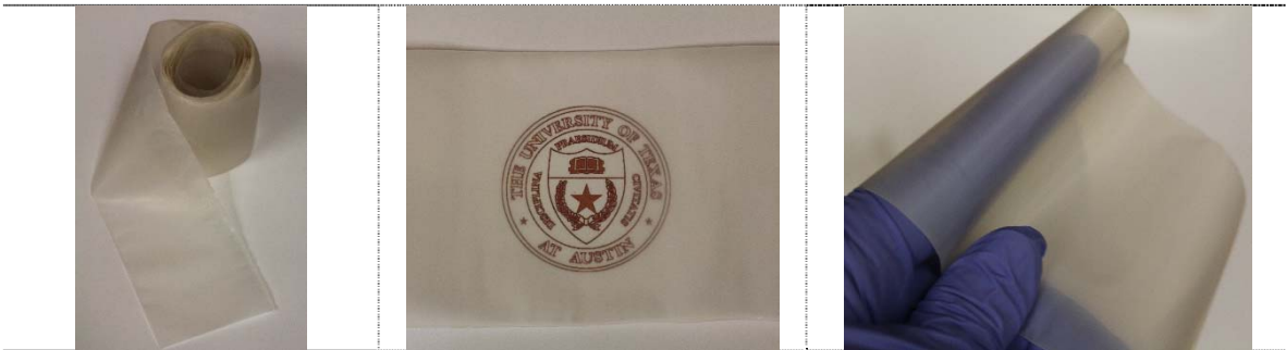
[c] BPS-20K ( \bar{M}_w = 31,300 g/mol)/PEG 300 20 wt% Extruded film
