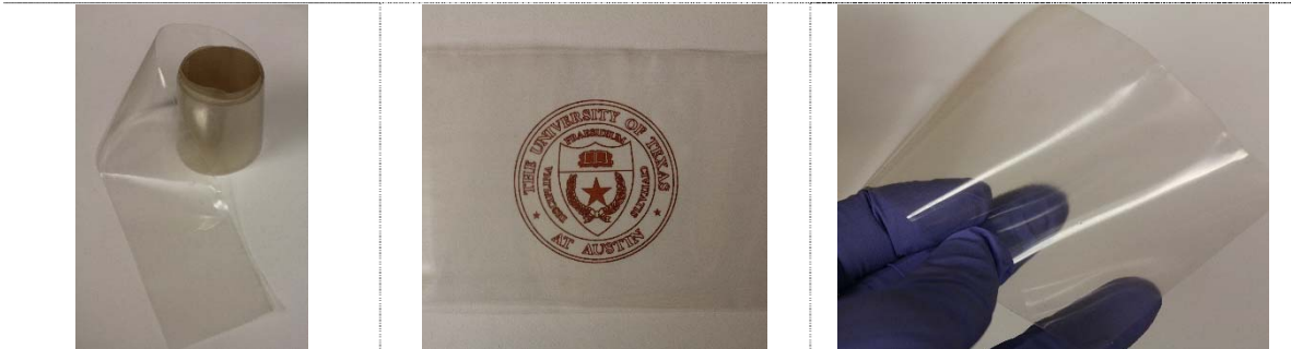
[d] BPS-20K ( \bar{M}_w = 31,300 g/mol)/PEG 400 20 wt% Extruded film
