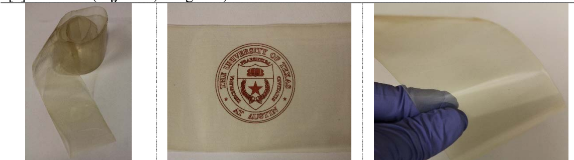
[c] BPS-20K ( \bar{M}_w = 39,000 g/mol)/PEG 200 30 wt% Extruded film
