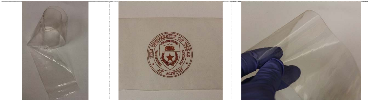
[f] BPS-20K ( \bar{M}_w = 31,300 g/mol)/PEG 200 30 wt% Extruded film
