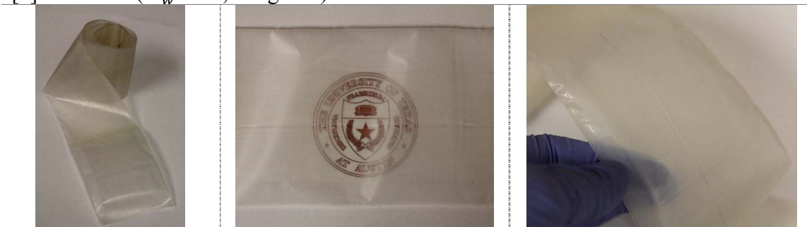
[c] BPS-20K ( \bar{M}_w = 39,000 g/mol)/PEG 200 30 wt% Extruded film
