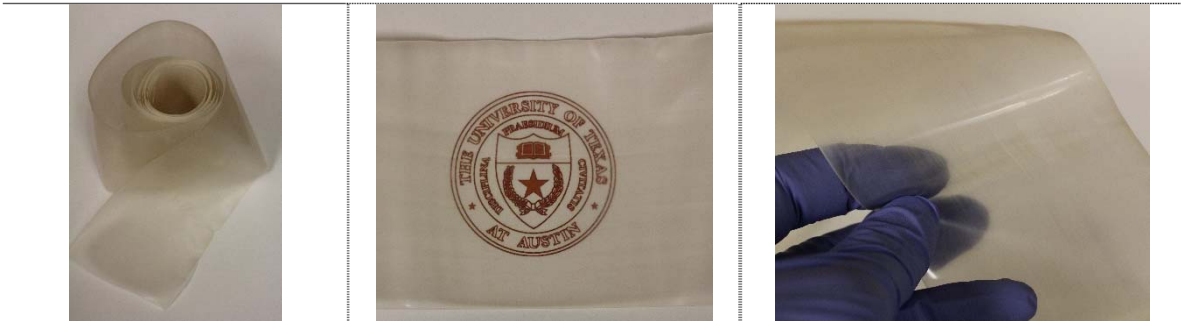
[d] BPS-20K ( \bar{M}_w = 31,300 g/mol)/PEG 400 20 wt% Extruded film
