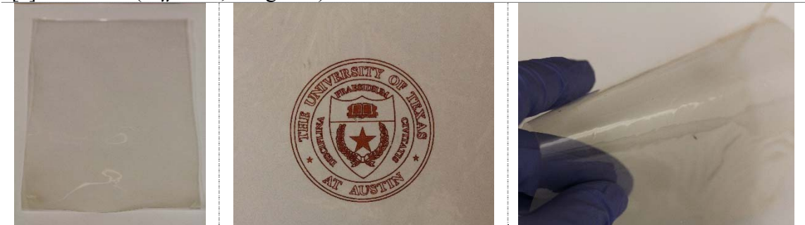
[b] BPS-20K ( \bar{M}_w = 39,000 g/mol)/PEG 200 20 wt% Extruded film
