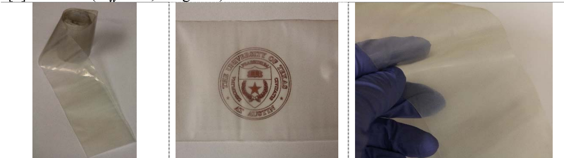
[b] BPS-20K ( \bar{M}_w = 33,200 g/mol)/PEG 200 20 wt% Extruded film
