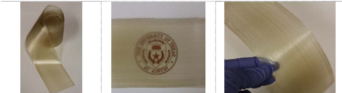
[f] BPS-20K ( \bar{M}_w = 31,300 g/mol)/PEG 200 30 wt% Extruded film
