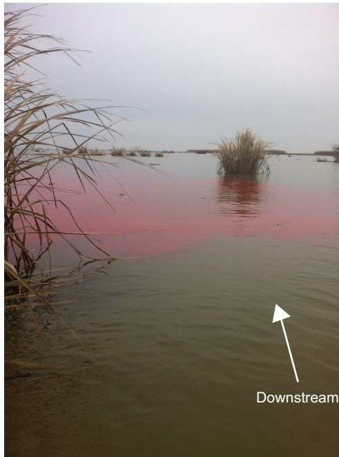
Figure 3.10: Image looking downstream taken 30 minutes after the rhodamine dye release on 02/07/2014. The rhodamine dye plume is bright pink due to high concentrations near the release point.
