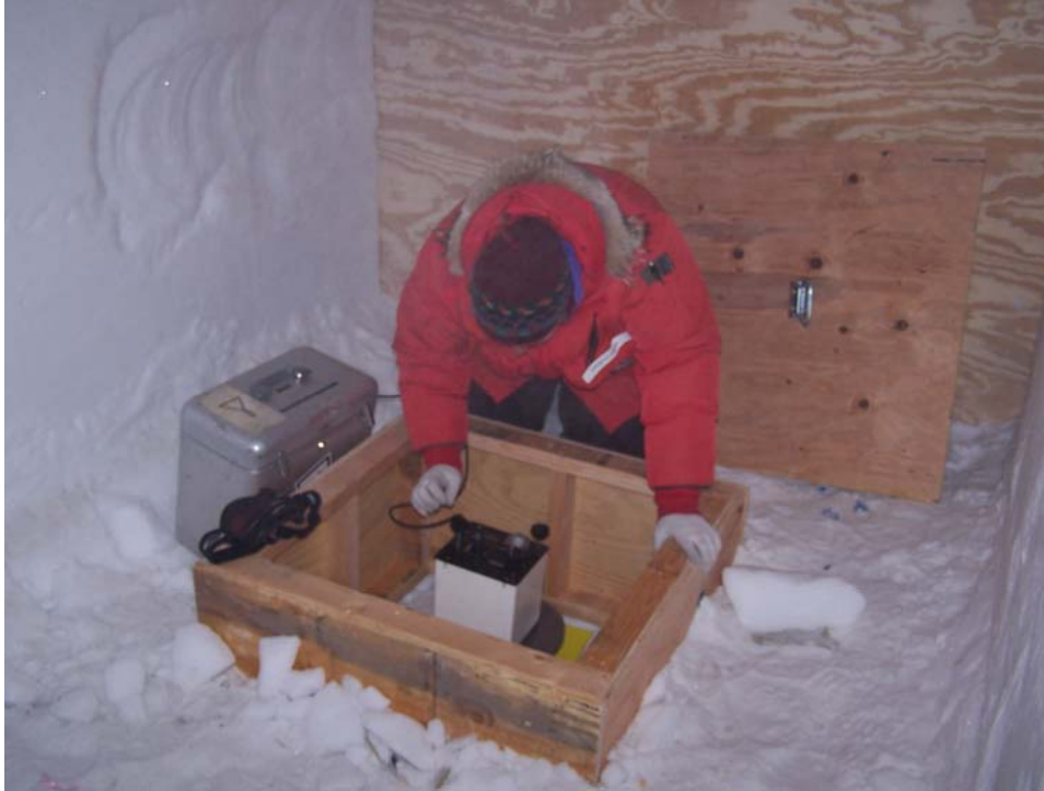
Figure 2.6: Theresa Diehl taking a gravity reading at the New South Pole station.
