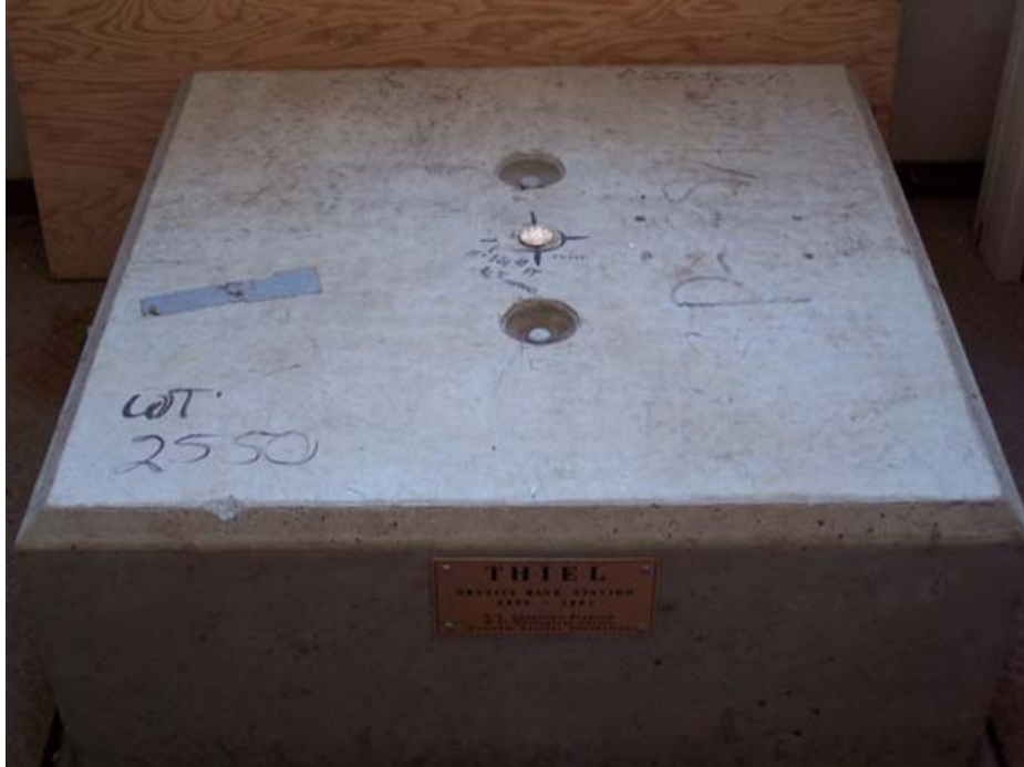
Figure 1.1: THIEL Gravity Benchmark in Bldg 146
