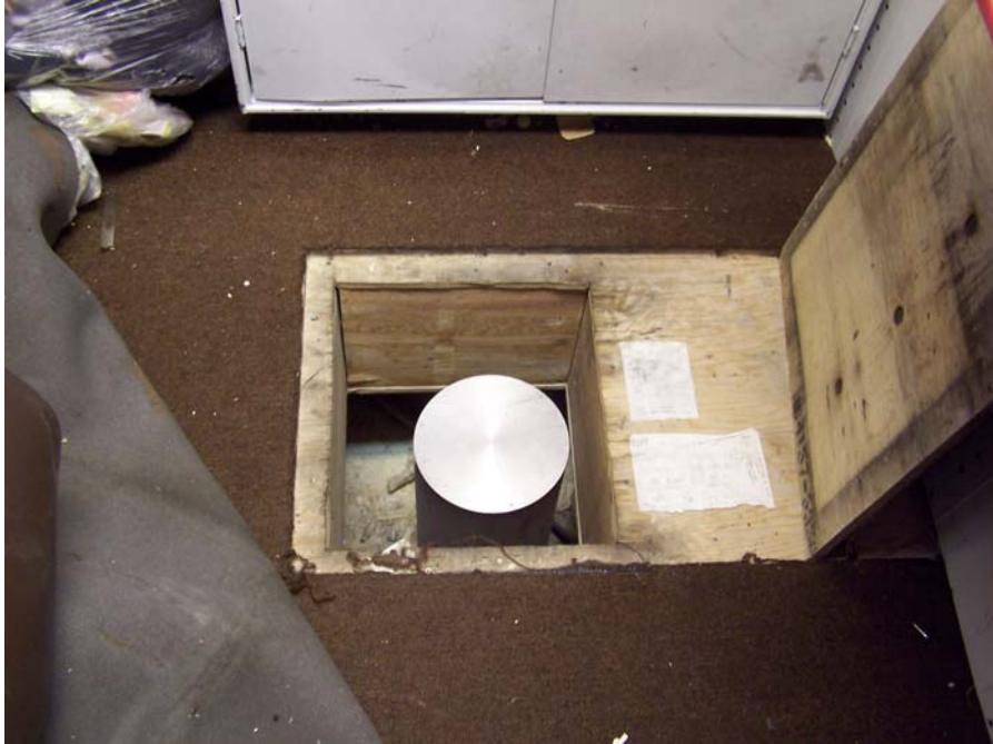
Figure 2.1: Metal pier gravity station below floor hatch in the South Pole Dome
