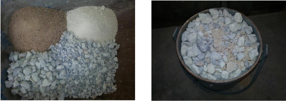
Figure 7.7 Coarse and fine aggregates before blending (left) and after blending (right) to determine DRUW. Theoretical cement paste volume was equal to the void content calculated from DRUW.
