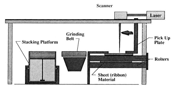
Figure 6: Laminated Object Manufacturing (LOM)
