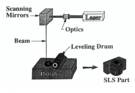
Figure 5: Selective Laser Sintering (SLS)
