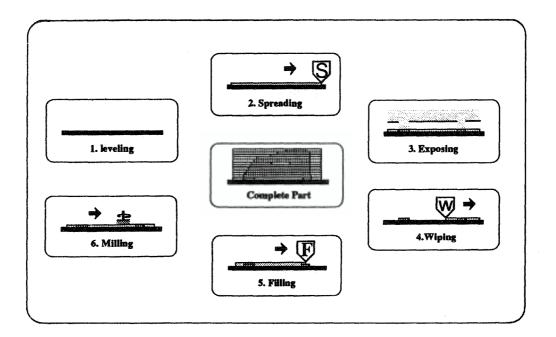
Figure 3: Cubital Instant Slice Curing Solider System
