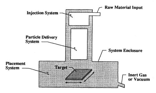
Figure 7: Ballistic Particle Manufacturing (BPM)
