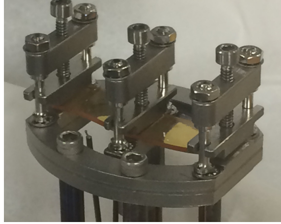
Figure 4.3: The double cantilever DMA experimental setup. The two external clamps are statically fixed, while a force is measured at the central clamp which moves at a controlled amplitude and frequency.
