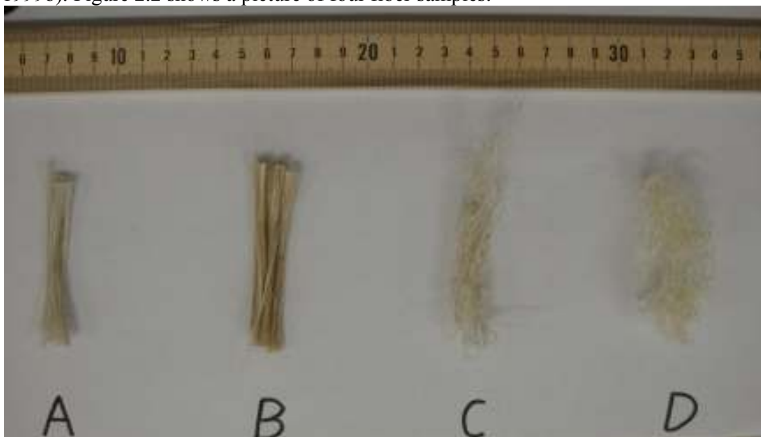
Figure 2.2 Pictures of four fibers: (A) kenaf (B) jute (C) raw sunn hemp (D) treated sunn hemp
