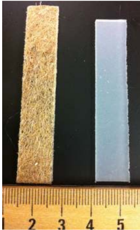
Figure 5.3 Specimens for DMA tests: (left) KPNC and (right) solid virgin PP
