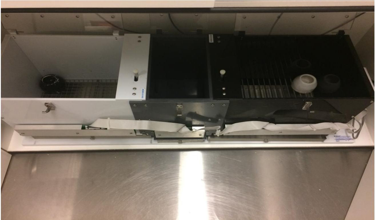
Figure 3. Photograph of CPP apparatus. Colored ceramic weights can be seen in rear of each compartment.
