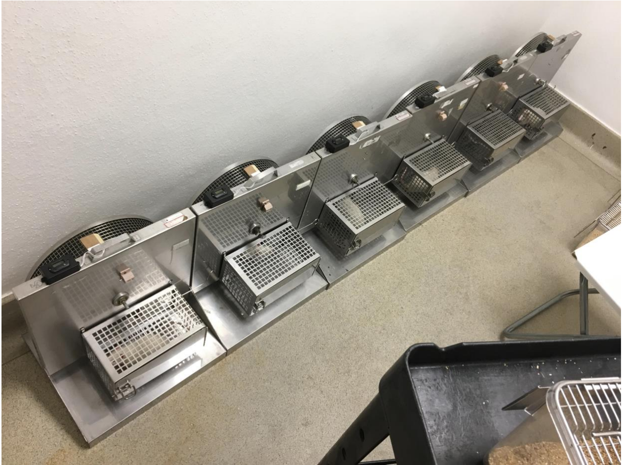
Figure 2. Free running wheels (rats in side compartment) used for voluntary exercise protocol.
