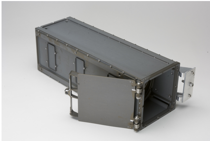
Figure 1.3: Cube satellite payload fairing and deployment structure called the P-POD[7].
