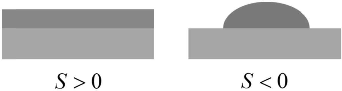
Figure 4. Schematic representation of the spreading parameter. The liquid forms a dome if the spreading parameter is negative.
