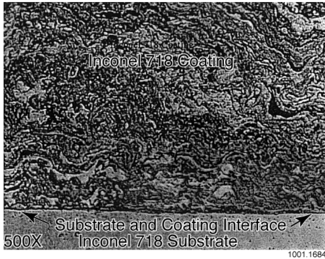
Fig. 1. EDP buildup coating
