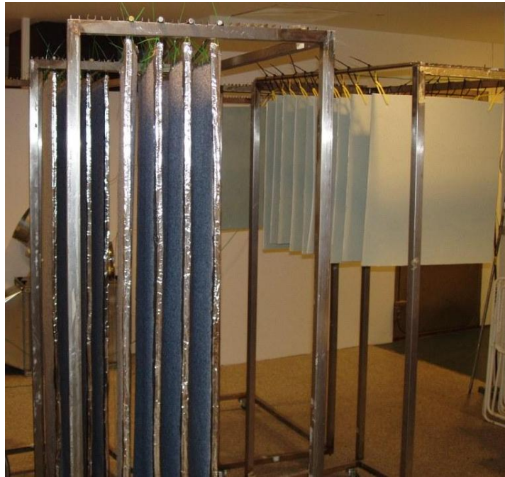
Figure D1. Configuration of carpet and clay plaster specimens on metal racks for PAQ analyses.
