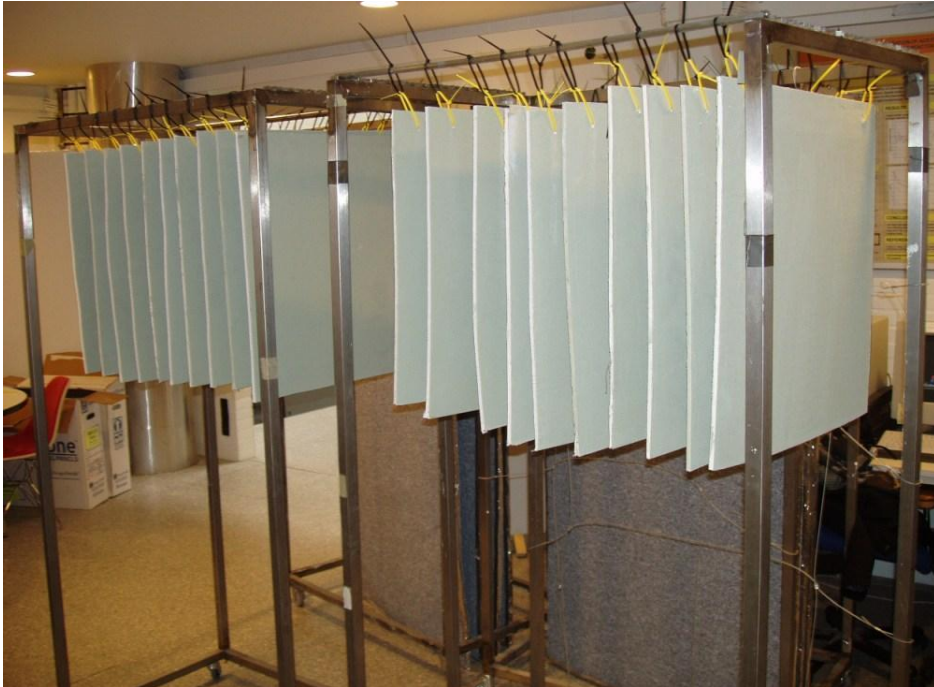
Figure D2. Configuration of clay plaster specimens on metal racks for PAQ analyses.
