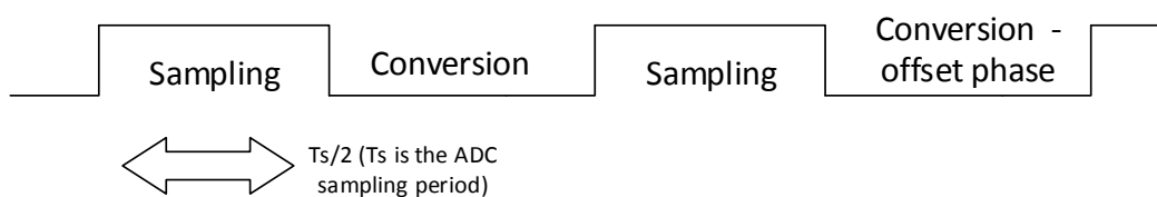
Figure 2.2: Interleaved ADC operation for the offset generation phase
