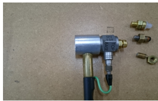
(b) Instrumented hammer with three varied stiffness tips and a force transducer.
