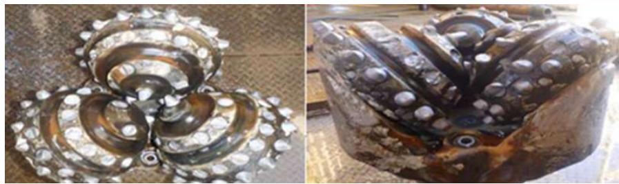
(a) Photos of the first bit showing significant damage.
