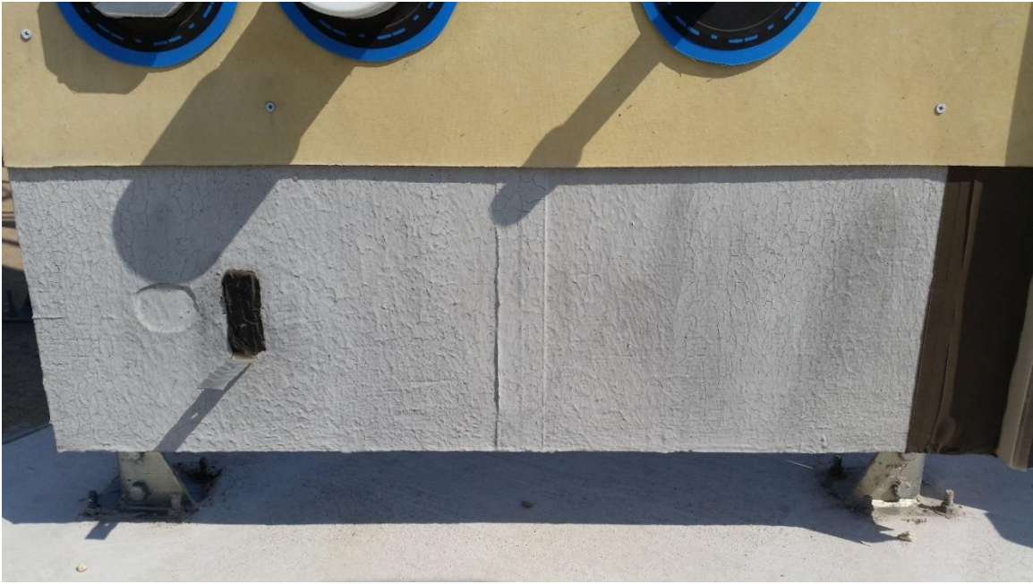
Figure 3.9: Specimen DRP1009-16 Crazing Observed After 3 Years of Exposure.
