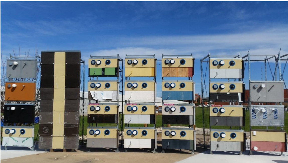
Figure 3.2: WRB Mockups at the Exposure Site.
