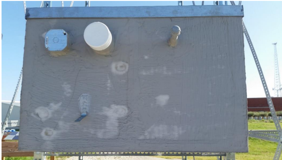
Figure 3.7: Specimen DRP1009-24 7 Months After Exposure Showing Discoloration.
