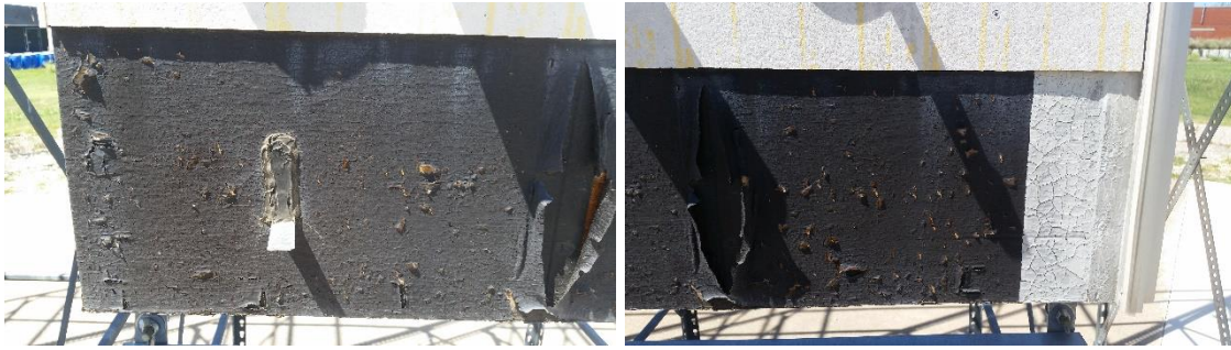
Figure 3.20: Tearing of Specimen DRP1009-09.
