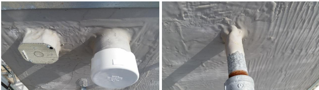
Figure 3.10: Pinholes Noted on Specimen DRP1009-24 Before the End of UV Permitted Exposure Time.
