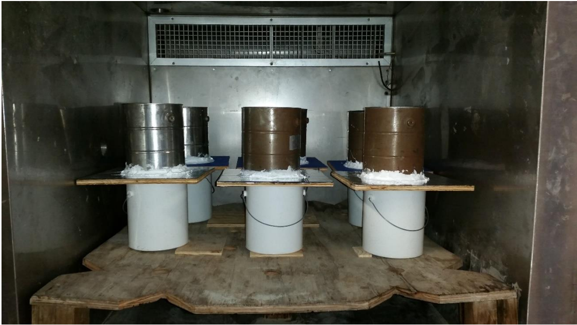
Figure 3.4: Test Assembly of Nail Sealability Testing.
