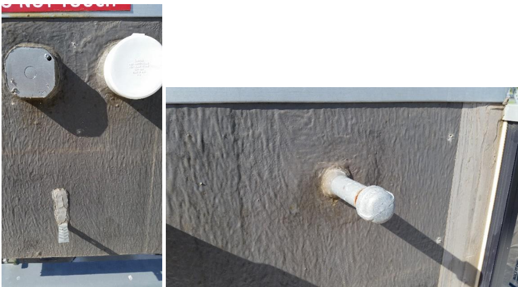
Figure 3.14: Dirt Pick Up of Specimen DRP1009-11 After Siding Removal 3 Years and 3 Months From Exposure.
