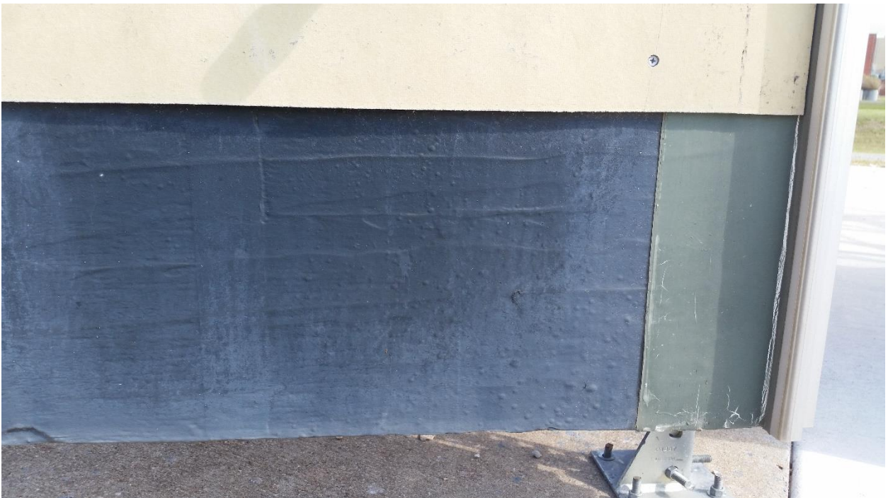
Figure 3.16: Specimen DRP1009-07 with a Great Number of Air Bubbles after 3 Years 9 Months of Exposure.
