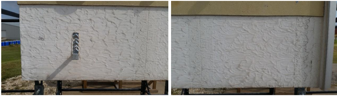
Figure 3.11: Specimen DRP1009-01 3 Years and 11 Months After Exposure.
