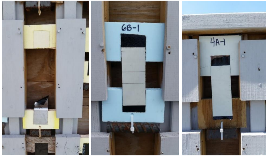
Figure 6.7: Vertical Sliding of the Scrim.
