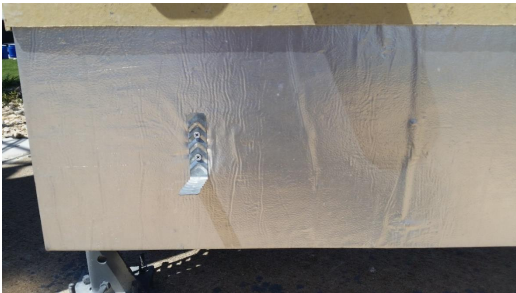
Figure 3.18: Specimen DRP1009-06 Vertical "Waves" Noted at the Uncovered Part 3 Years 3 Months After Exposure.
