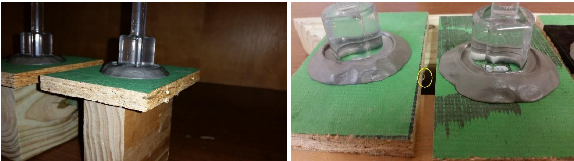
Figure 3.24: Water Falling From the Edges of the Sheathing.
