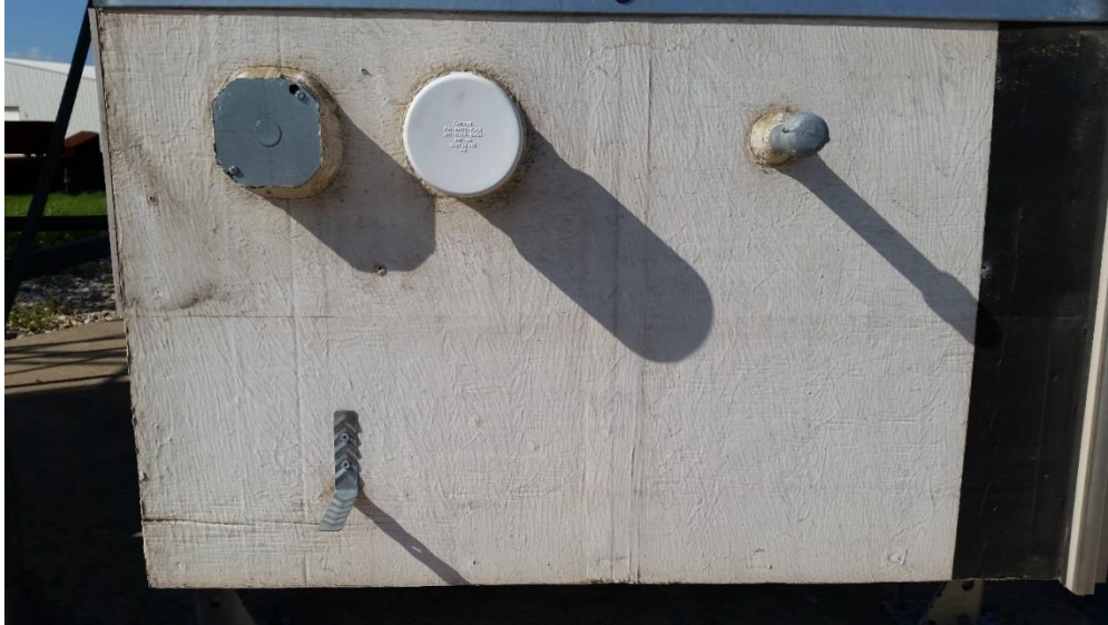
Figure 3.14: Dirt Pick Up of Specimen DRP1009-11 After Siding Removal 3 Years and 3 Months From Exposure.
