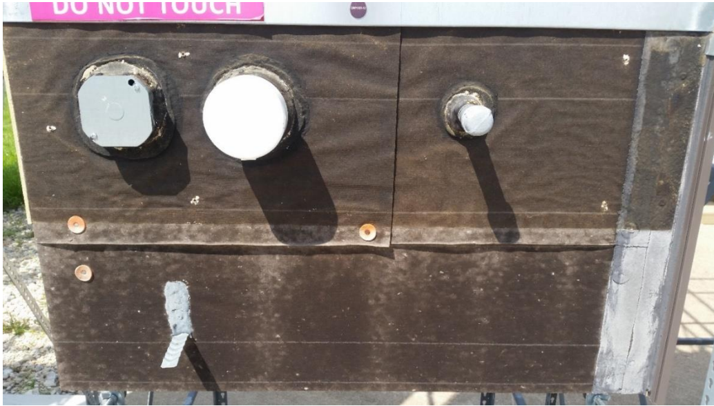
Figure 3.17: Specimen DRP1009-12 Waviness at Covered Part.
