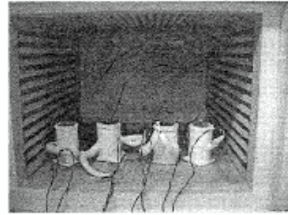
Figure 7 Samples mounted with strain gauges in a temperature controlled oven.
