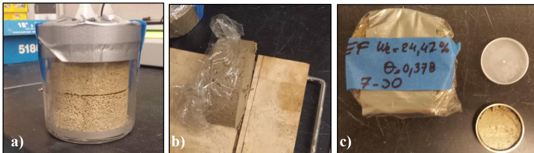
Figure 10. (a) Sample in the glass container, (b) slicing, and (c) set in WP4C bin.
