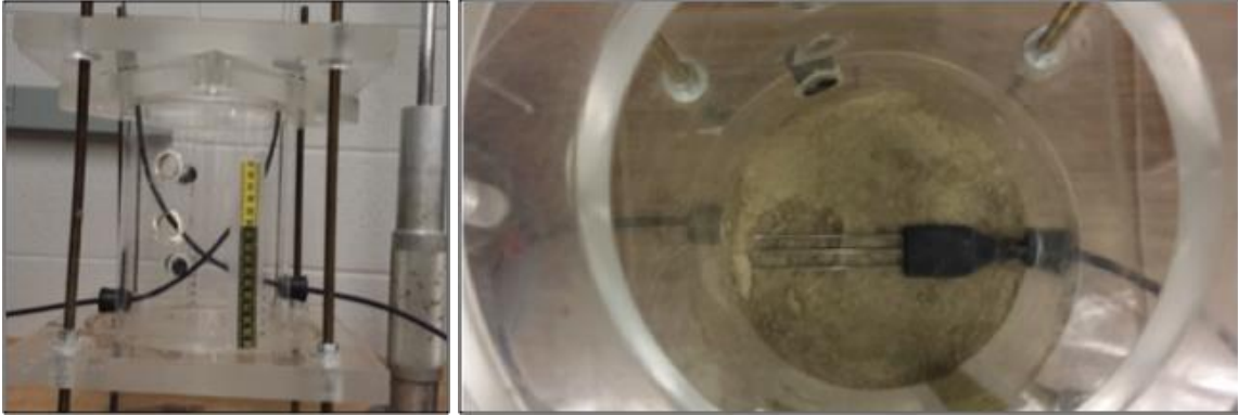
Figure 156. Column set up for Eagle Ford calibration: a) lateral view before placing soil, and b) top view during compaction procedure.
