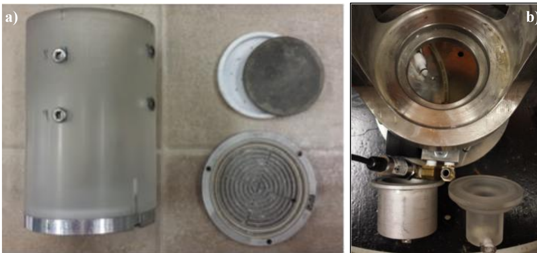
Figure 12. Lower boundary of the centrifuge permeameter cups: a) aluminum base, and b) outflow instrumented with a pressure transducer.
