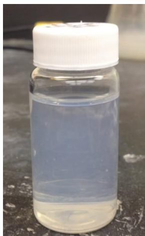
Figure 3.16 IPA-ST nanoparticle dispersion. The nanoparticle dispersion is 2 wt.% IPA-ST nanoparticles and 3 wt.% NaCl.
