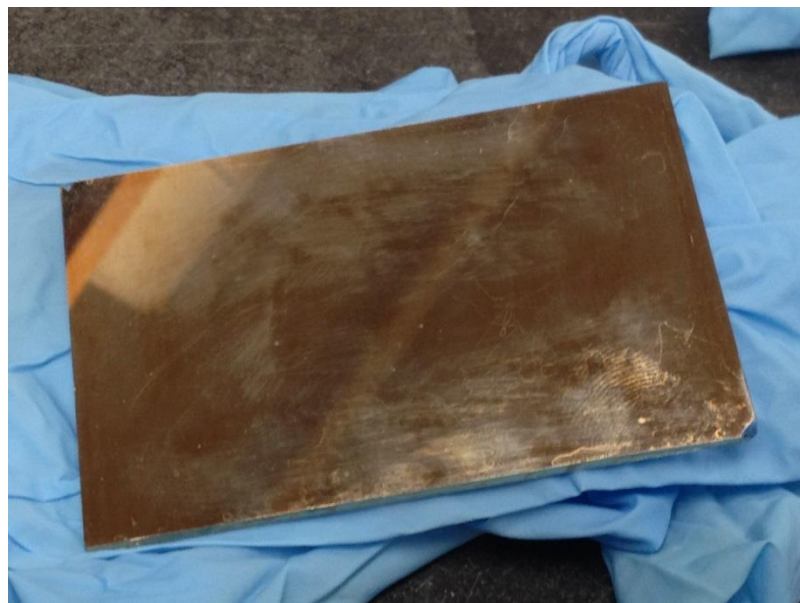
Figure 3.11 Copper backed mirror after treatment with methylene chloride
