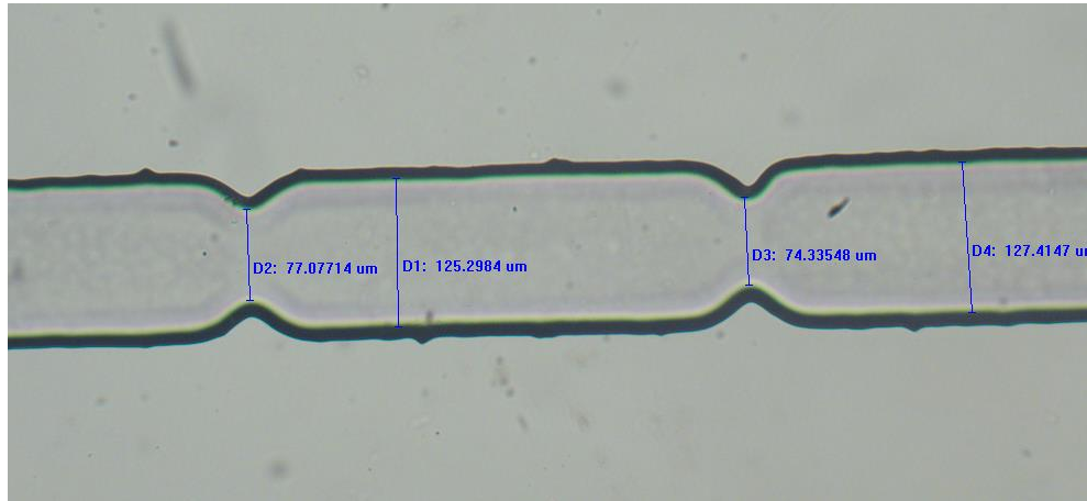
Figure 3.15 Etched profile of a converging-diverging pore space. The profile is more uniform than the procedure used to create dead-end pore channels.
